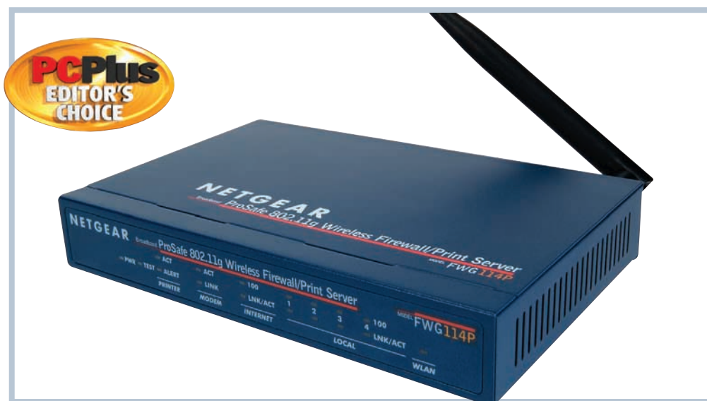
Clothed in Netgear's standard blue chassis, the FWG114P offers a quad of switched, dual-speed Ethernet ports, while a separate port is provided for the WAN connection.
