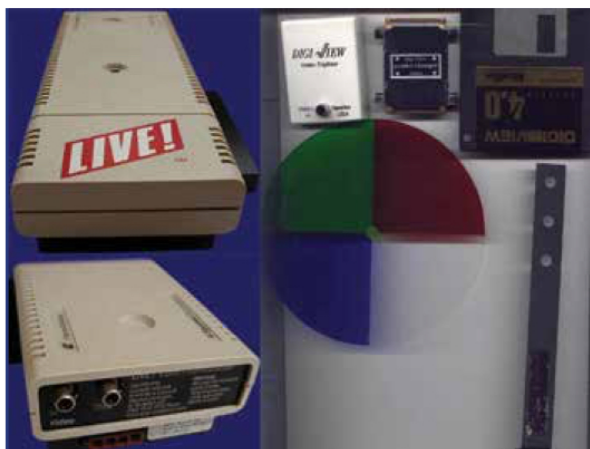
A couple of digitizers for the Amiga computer from the late 1980s. On the left, Live by A-squared and on the right, Digi-View from NewTek, showing the color wheel you had to shoot through
