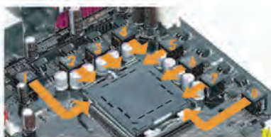
8-phase design operate at 15°C lower than conventional power solution
