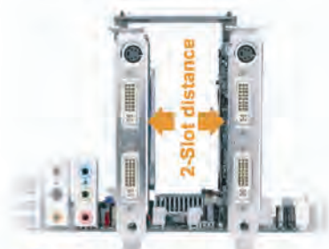
2-Slot distance : Provides better airflow to ensure reliable system stability
