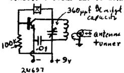
I KEYED THE 8- LEAD USUALLY, AND THE RIG FOLLOWED A BUG NICELY. THE ENTIRE RIG, WITH A 9 VOLT BATTERY, IS BUILT IN A 'SUCRETES' LOZENGE BOX. THE TANK COIL WAS WOUND ON AN IRON CORE FORM, AND THE TURNS WERE ADJUSTED TO RESONATE AT 3.5 MC AT ABOUT THE 150MMF SETTING OF THE TANK CAPACITOR. THE LINK COIL WAS 3 OR 4 TURNS. THIS CIRCUIT IS ONLY A NOVELTY AS NO PROTECTION IS GIVEN TO THE TRAN-SISTOR. I'VE POPPED SEVERAL TRANSITORS
