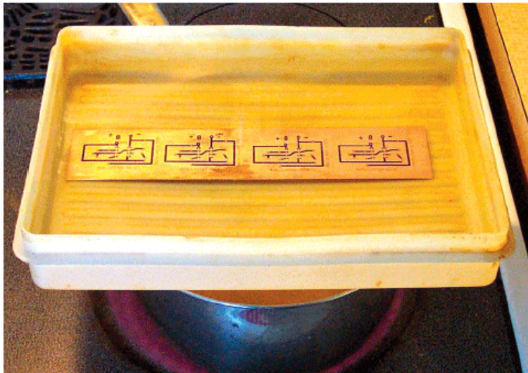
Etch the PCB on the stove.
