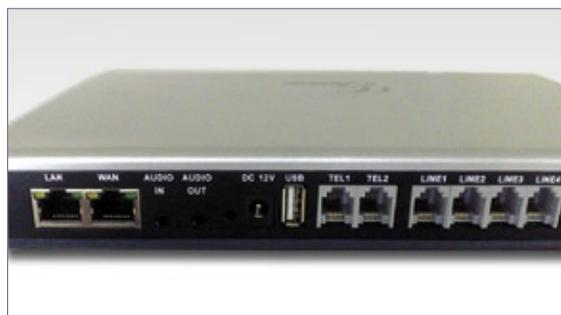
Figura 1 No painel traseiro do aparelho, as portas Ethernet, FXO, FXS e USB.
