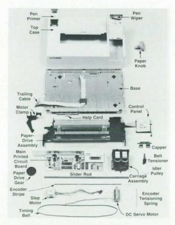
Fig. 3. Exploded view of the PaintJet printer.
