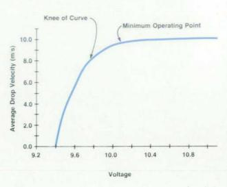
Fig. 2. Typical result of an operating window test of a printhead.
