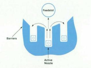
Fig. 8. Diagram showing three nozzles, the ink feedslot, and the fluid barriers. Hydraulic cross talk consists of ink flow back down the barriers to the feedslot and to neighboring nozzles. slowed enough to cause the drop ejection to be on top of the first overshoot in some situations. To compensate for this, it was decided to increase the barrier height, which decreases the fluid drag in the channel, resulting in faster refill.
