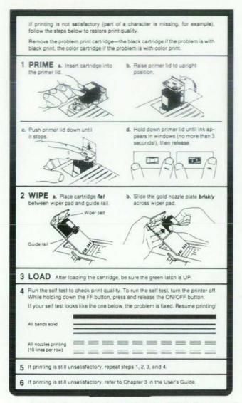
Fig. 10. The primer allows the user to activate the pen and correct printing problems. These instructions are on a pull-out card attached to the printer.
