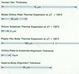
Fig. 1. Comparison of notable thermal inkjet physical dimensions to the thickness of a human hair.
