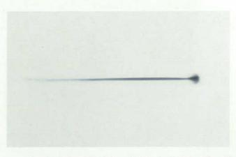
Fig. 5. Photograph of drop ejection. The length of the tail depends on the ejection velocity.
