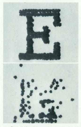
Fig. 1. Misinformed character (bottom) resulting from soft plug formation. The top photo shows the character as it should look.
