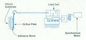
Fig. 6. Peel tester used in the adhesive tests.
