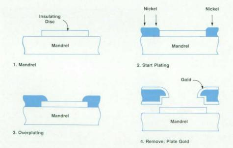
Fig. 5. Orifice plate electroforming process.
