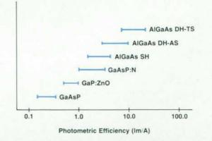
Fig. 5. Photometric efficiency ranges for plastic lamps made with the different red LED chips at a forward current of 20 mA.
