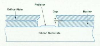
Fig. 4. Small gaps between the orifice plate and the substrate caused reduced and irregular drop velocities. A new process eliminates them. (Not drawn to scale.)
