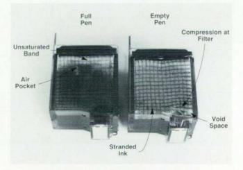
Fig. 1. Clear-bodied full and empty PaintJet printer pens (print cartridges), showing foam ink reservoir.
