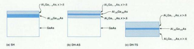
Fig. 3. The three types of red AlGaAs LEDs that are commercially available.
