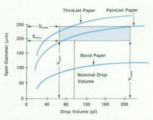
Fig. 4. Spot diameter as a function of drop volume for the PaintJet printer ink/paper system, with other papers shown for comparison.
