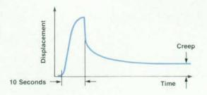
Fig. 9. Typical creep shear test result.
