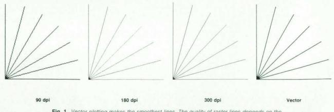
Fig. 1. Vector plotting makes the smoothest lines. The quality of raster lines depends on the resolution.
