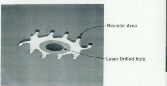
Fig. 3. In the PaintJet color cartridge, each group of ten resistors is supplied with ink through a laser-drilled hole.
