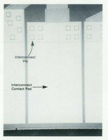
Fig. 2. Contact pads on the printhead are connected to conducting traces by multiple interconnect vias.
