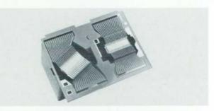
Fig. 7. A leadframe in contact with print cartridges.
