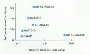
**Fig. 7.** Typical performance-to-cost ratio in mcd per unit cost versus relative lamp cost for all of the red LED technologies. Lamps with a viewing angle of 24 degrees measured at 20 mA were used to generate the mcd values.
