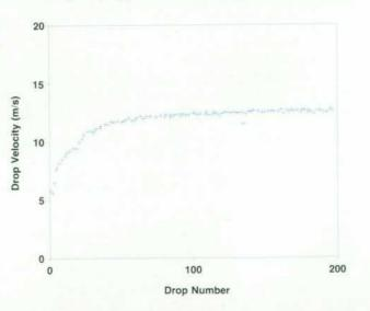
Fig. 9. Startup plot for a pen that has been inactive for several minutes. Drop velocity increases as high-viscosity ink is purged from the nozzle. In the PaintJet printer, these slow drops are purged before printing begins.
