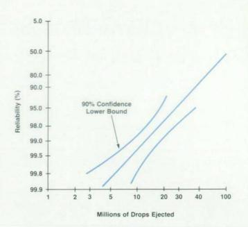
Fig. 8. Weibull plot for printheads.
