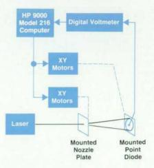
Fig. 6. System for measuring orifice plate nozzle diameters to an accuracy of  $\pm 0.5 \ \mu m$ .
