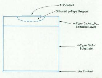
Fig. 1. Structure of a typical homojunction GaAsP LED. The pn junction is formed by a Zn diffusion into an n-type GaAsP epitaxial layer. Light is generated on both sides of the pn junction and escapes primarily from the top surface.
