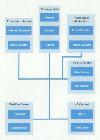
Fig. 1. Block diagram of the custom CMOS IC in the HP PaintJet Color Graphics Printer. up the swath buffer, each of the 30 bit rows of a character needs to be "pasted" to the previous characters in the buffer. Since our RAM is organized in bytes, a bit-map row may have to be shifted before pasting, to maintain byte alignment. The worst case is a seven-dot shift, requiring a three-byte (fifteen dots plus seven dots) shifter.
