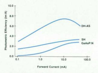
Fig. 4. Photometric efficiency in lumens/ampere versus forward current for typical SH and DH-AS AlGaAs LED lamps. Also shown for comparison is the curve for a typical GaAsP:N lamp. GaAsP:N now dominates the high-performance, highvolume market.
