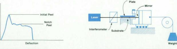
Fig. 7. Typical data from a peel test.
