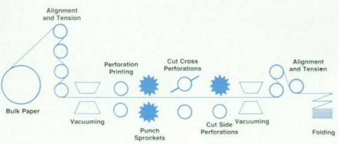
Fig. 5. PaintJet printer paper conversion press schematic diagram.
