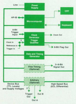
Fig. 3. HP 8175A block diagram.
