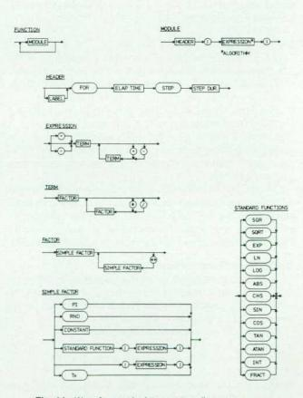
Fig. 11. Waveform calculator syntax diagrams.
