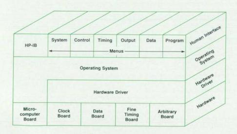
Fig. 2. HP 8175A system architecture has four layers, three software and one hardware.
