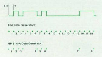
Fig. 8. A traditional data generator needs 18 memory locations for the data stream illustrated. The HP 8175A has variable timing and needs only eight.
