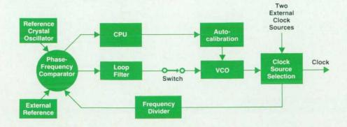
Fig. 12. For phase-locked operation, the delay-line oscillator is embedded in a standard phaselocked loop.
