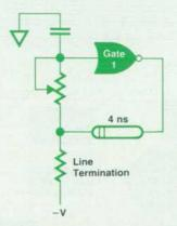
Fig. 10. Delay-line oscillator has an adjustment for gate delay variations.
