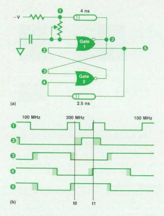
Fig. 11. Flip-flop circuit prevents third-harmonic oscillations.
