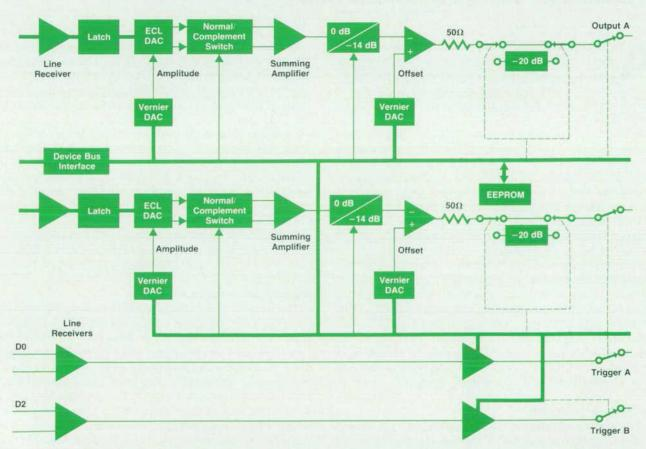
Fig. 15. Arbitrary waveform generator functional block diagram.
