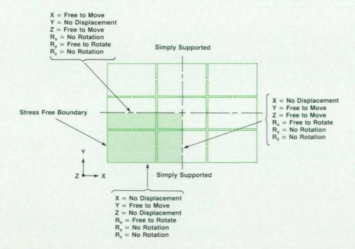
Fig. 3. Displacement boundary conditions.
