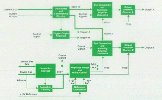
Fig. 14. Arbitrary board block diagram.
