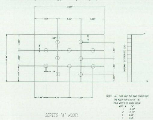
Fig. 2. Model of a partially routed printed circuit board panel with a uniform load.
