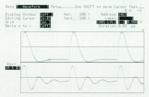
Fig. 7. The physical screen can be divided vertically into as many as four logical screens.
