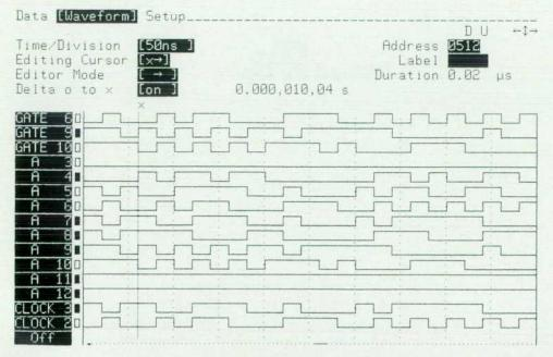
Fig. 5. Graphic display for the data generator configuration.
