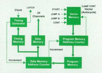
Fig. 6. Data board block diagram.
