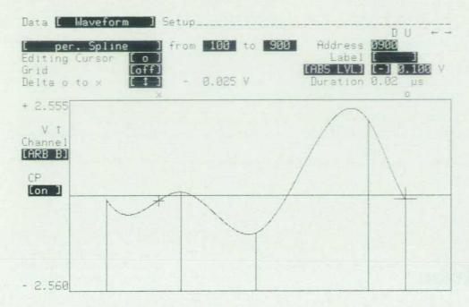
Fig. 8. Waveforms that are impractical to describe mathematically can be simulated by entering characteristic points.
