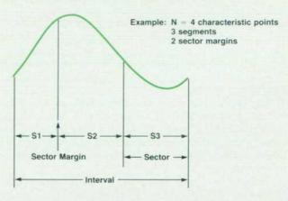
Fig. 9. Third-order polynomial interpolation is done between characteristic points.
