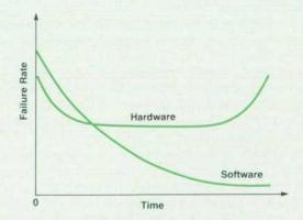
Fig. 1. Characteristic failure rate curves
