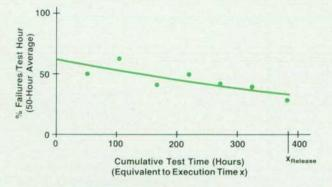
Fig. 3. HP 2394A prerelease failure rate
