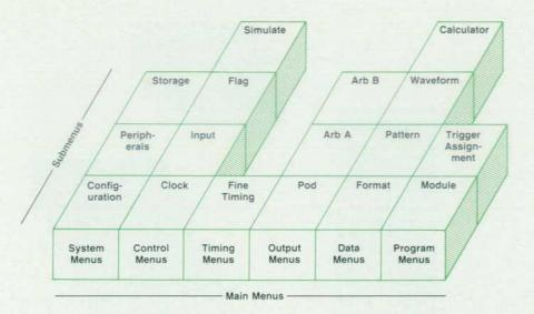
Fig. 1. The user interface of the HP 8175A Data Generator distributes all instrument settings over six main display pages, or menus.
