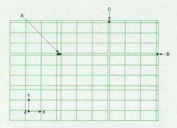
Fig. 4. Finite element model for the partially routed panel. Elements A, B, and C refer to Figs. 8 and 9.
