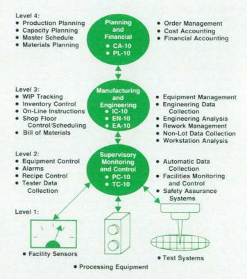
Fig. 2. HP's Semiconductor Productivity Network is a collection of hardware and software products designed to aid microelectronic product fabrication personnel in controlling, monitoring, improving, and managing many of the levels of the complex manufacturing process.
