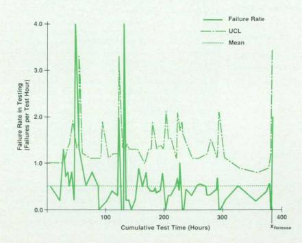
Fig. 4. HP 2394A testing process control chart.
