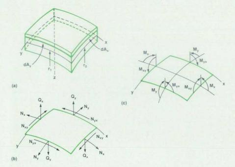
Fig. 5. Forces and moments acting on a thick-shell element.
