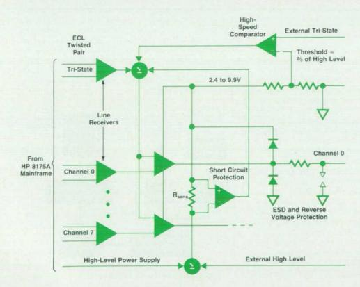
Fig. 4. Diagram of the TTL/CMOS pod. This pod provides for control of its output high level by the user or by the device under test.
