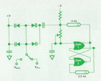
Fig. 13. A varicap diode circuit provides a controllable frequency range of ±2.4 MHz at 100 MHz.
