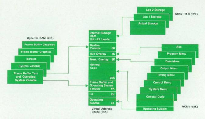
Fig. 3. Typical HP 8175A internal memory allocations.
