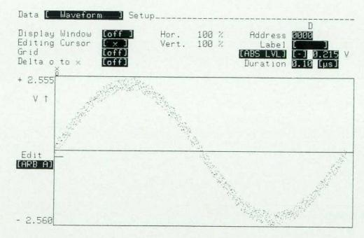
Fig. 15. The result of combining noise and a sine wave.
