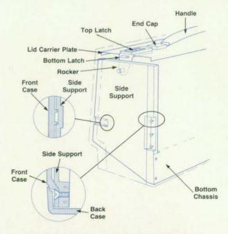
Fig. 2. Details of handle and side support assemblies.
