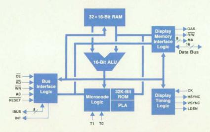
Fig. 1. Block diagram of custom graphics processor unit for the Integral PC.
