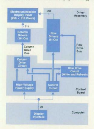
Fig. 2. Block diagram of Integral PC display system.
