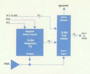
Fig. 3. Block diagram of memory management unit.
