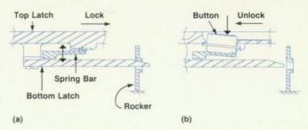
Fig. 4. Latch operation. (a) Locking, edge cross section of mechanism (button not shown). (b) Unlocking, center-line cross-section of mechanism showing caged release button. See Fig. 2 for perspective view.
