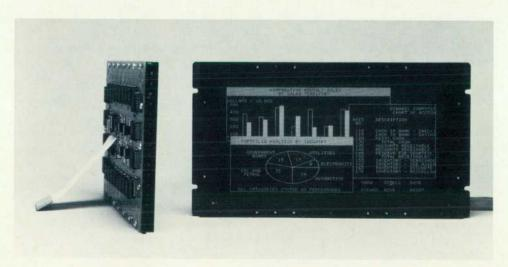
Fig. 1. Commercially available 256×512-pixel electroluminescent display.
