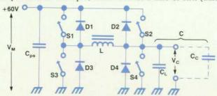
Fig. 8. Equivalent circuit for the column drive used for the Integral PC display (see text for explanation of its operation).
