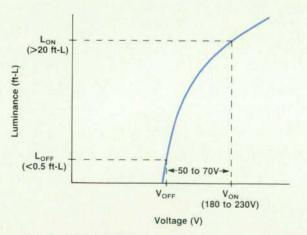
Fig. 4. Typical luminance-versus-voltage curve for electroluminescent display.
