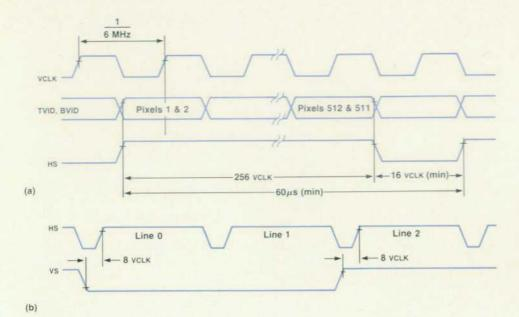
Fig. 11. Timing diagrams for interface signals between the display system and the rest of the Integral PC electronics. (a) Horizontal sync versus video clock and pixel enables. (b) Horizontal sync versus vertical sync.
