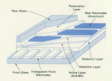
Fig. 3. Structure of electroluminescent display panel.
