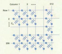
Fig. 7. Each pixel of the electroluminescent display contributes a capacitance C<sub>e</sub> that must be charged and discharged by the driver ICs.
