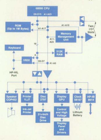
Fig. 1. Block diagram of electronics system for the Integral PC.
