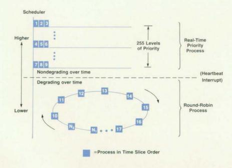
Fig. 4. Real-time priority and scheduling scheme used in the Integral PC operating system.
