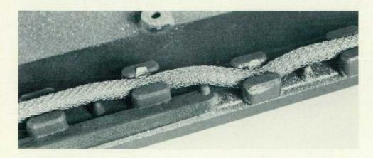
Fig. 4. The conductive rope gasket used to seal the Model 520's enclosure against EMI is located between the case halves and retained in place by ultrasonically deforming two parallel rows of oval bosses as shown. The triangular ramps ensure conductive contact between the case halves.
