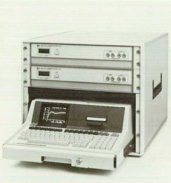
Fig. 1. A powerful, compact, yet low-cost data acquisition system, the HP 3056DL, is formed by combining one or more 3421As with an HP-85 Computer.
