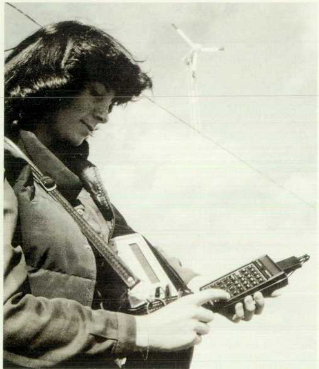
Fig. 3. Measuring electrical parameters in the field is now much easier using a 3468A Multimeter, an HP-41 Handheld Computer, and the 44468A DA/C Pac ROM.
