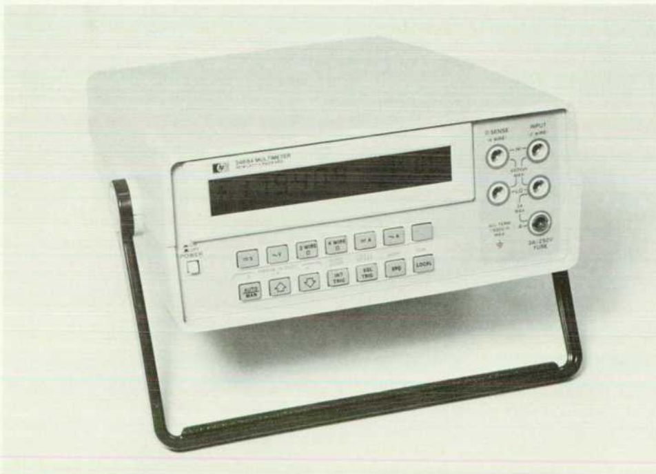
Fig. 1. The HP Model 3468A Multimeter is HP's first HP-IL instrument. It has an alphanumeric liquid-crystal display, measures ac and dc voltage and current, and determines resistance by both two-wire and four-wire methods.
