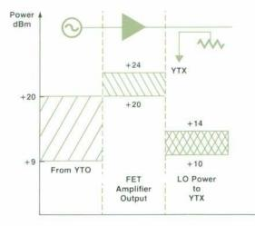
Fig. 4. Variations in the local oscillator power supplied to the mixer diode are compressed by operating the FET amplifier in a saturated mode.
