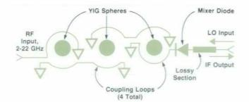
Fig. 2. Schematic representation of the YIG-tuned filter and mixer (YTX) used in the 8566A. Although this shows all the coupling loops in the same plane, the two loops for each YIG sphere cross at an angle so coupling occurs only at the resonant frequency of the YIG sphere, which is a function of the dc magnetic field strength.
