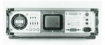
**Fig. 8.** The ENABLE SELECT switches and two of the four ENABLE inputs are on the rear panel. Also on the rear panel are the LOGIC POLARITY switches, DAV DELAY Adjustment, RS 232C BAUD RATE select, and HP-IB addresses (KEYBOARD and DATA MODES).
