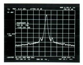
Fig. 2. Spectrum display of an 18-GHz signal made by the Model 8566A Spectrum Analyzer with a 10-Hz resolution bandwidth across a frequency scan of 600 Hz. The  $\Delta$  marker (rightmost brightened dot) is positioned on a 60-Hz line-related sideband that is 50 dB below the carrier. Until now, this high degree of resolution, made possible by the low phase noise and 10-Hz resolution bandwidth of the 8566A, had not been available in microwave spectrum analyzers.
