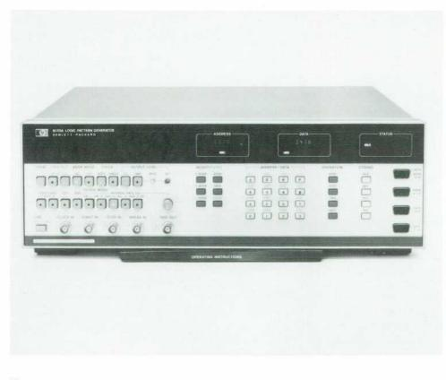
Fig. 1. Model 8170A Logic Pattern Generator produces long sequences of 8-or 16-bit parallel digital words as bus stimuli for functional tests of multichannel digital hardware. It operates at clock rates up to 2 MHz, internally or externally supplied.
