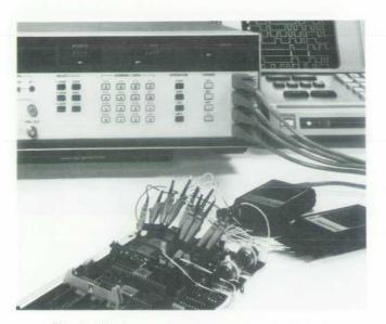
Fig. 2. Miniature probes like those used with logic state analyzers facilitate hook-up to the system being tested.
