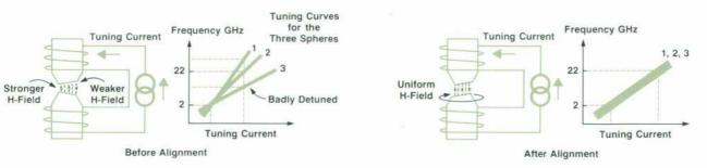
Fig. 3. Misalignment of the tuning magnet pole faces, shown exaggerated here, causes the three YIG spheres to have different tuning characteristics. Rotating the pole pieces to bring the tilted faces into parallel alignment achieves identical tuning characteristics for the three spheres.
