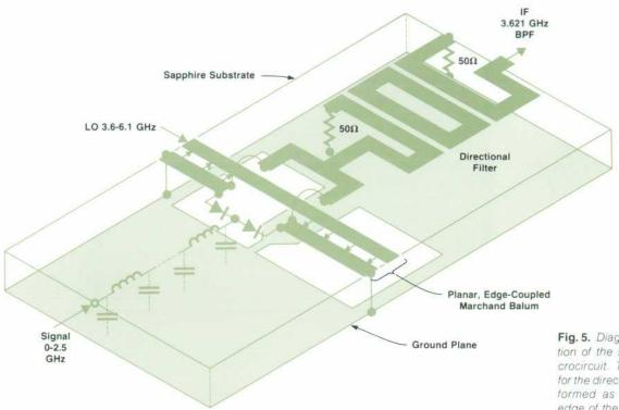
Fig. 5. Diagrammatic representation of the second converter microcircuit. The  $50\Omega$  terminations for the directional filter are actually formed as thin films along the edge of the substrate.
