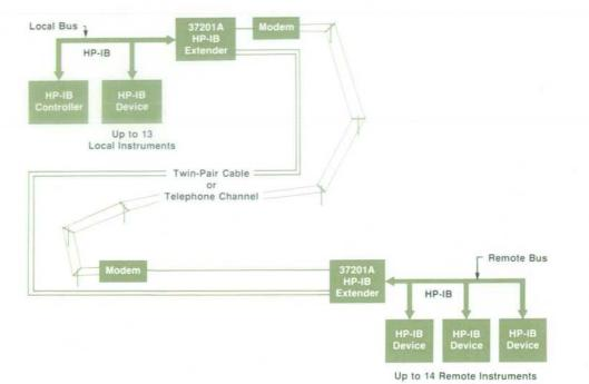
Fig. 2. Two distant clusters of instruments are connected through a pair of 37201A HP-IB Extenders in this basic configuration. The controller can communicate with the remote instruments as though they were connected to the local bus.
