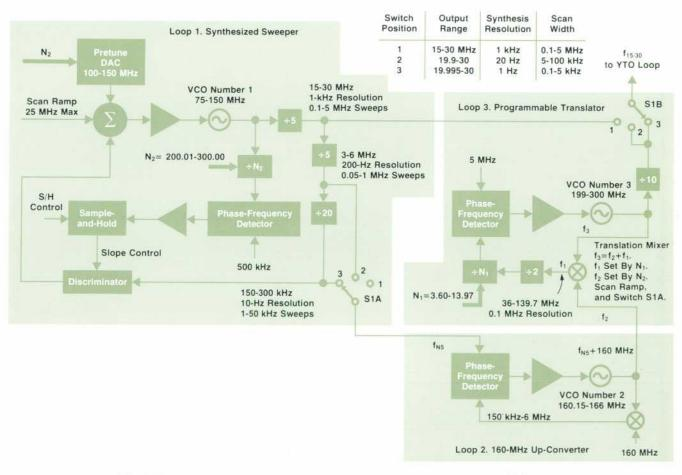
Fig. 4. The low-frequency synthesizer has three loops. Loop 1 is the basic source of a frequency that is divided down then up-converted by loop 2 and translated by loop 3 to derive an appropriate frequency for control of the YTO.
