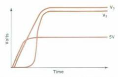
Fig. 4. Turn-on sequencing is designed for proper operation of semiconductor memory devices.
