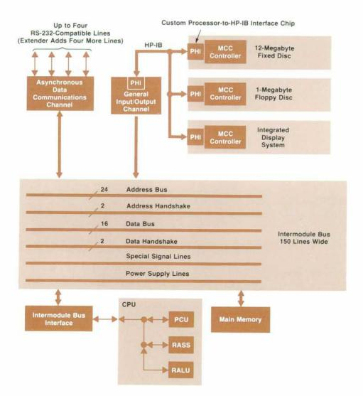
Fig. 4. The 150-line intermodule bus connects the processor elements, the memory elements, and the input/output channels. The bus is asynchronous and provides separate address and data handshake lines for better performance. Peripheral devices are connected to the general input/output channel via the HP Interface Bus (IEEE 488).
