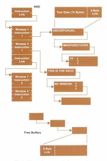
**Fig. 2.** IDS controller creates a display program in response to the user's window requirements. The program, organized as shown here, consists of a series of four-byte instructions and text. Text is stored as a series of linked 18-byte buffers.
