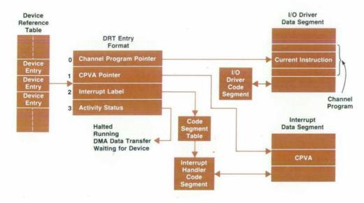
Fig. 1. HP 300 hardware input/ output system memory organization. Every I/O device has an entry in the device reference table (DRT). The channel program variable area (CPVA) contains interrupt parameters.
