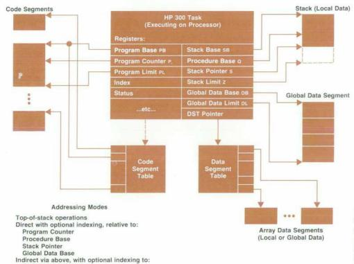
Fig. 1. HP 300 addressing scheme. The environment of an executing program includes non-modifiable code segments and a number of data spaces that include the stack, the global data segment, and array data segments as needed.
