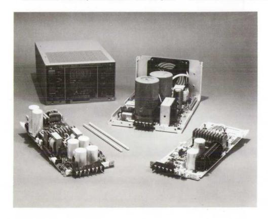
Fig. 1. Three interlocking, functionally independent printed circuit boards contain all the circuits in the 63312F Multiple Output Switching Power Supply. The supply provides up to 550 watts at 5V, ±12V or ±15V, and up to 40V.
