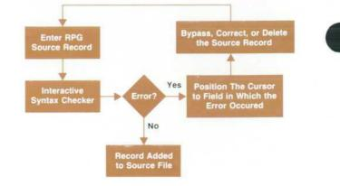
Fig. 7. RPG-II/300 detects syntax errors immediately so they can be corrected interactively.
