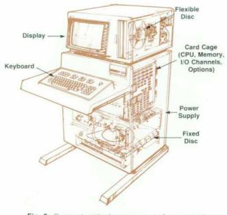
Fig. 2. Compact vertical arrangement of components conserves space in the office environment.
