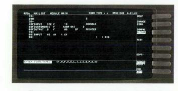
Fig. 3. To switch templates the user presses the CHANGEFORM softkey, and is offered a menu of form types.
