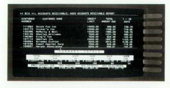
Fig. 3. The IDS screen can be divided into independent windows, each of which acts like a separate display. Windows are indicated by dotted-line borders on the screen.
