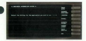
Fig. 2. Eight keys at the right side of the HP 300's integrated display system (IDS) can be assigned functions dynamically by application programs. The functions are displayed in a window next to these softkeys.
