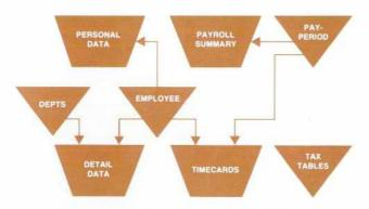
Fig. 3. An IMAGE/300 data base consists of a network of related master data sets (EMPLOYEE, PAY-PERIOD) and detail data sets (TIMECARDS).
