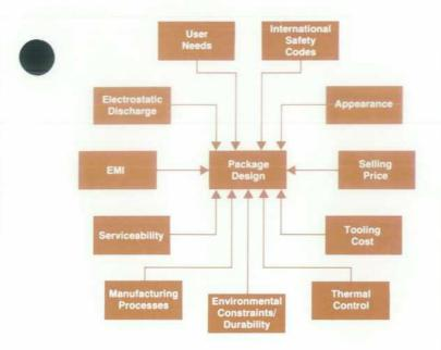
Fig. 1. Design parameters for the HP 300 package design.
