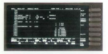
Fig. 4. Editing a previously entered line using the APPENDI MODIFY, SELECT LINE, and DELETE softkeys.
