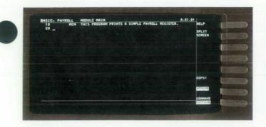
Fig. 4. BASIC language subsystem prompting for a new line of text illustrates typical use of the integrated display system (IDS) for program editing.
