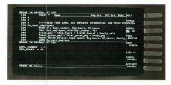
Fig. 8. Using the symbolic debug facility.
