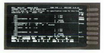
Fig. 5. When the TEST softkey is pressed, compilation begins. If an error is discovered, it is displayed on a split screen. The user can correct the error, BYPASS it temporarily, or our the error processing mode.
