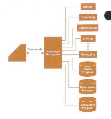
Fig. 2. HP 300 program development is simplified by the language subsystem concept.
