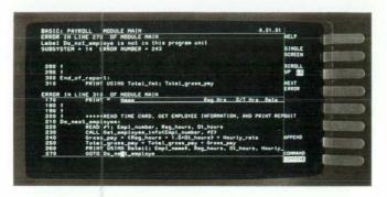
Fig. 7. Post-compilation error correction using the splitscreen feature and the NEXT ERROR softkey.
