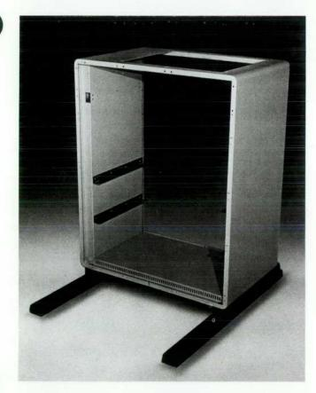
**Fig. 5.** The HP 300's skin serves as both cover and structure. This "minirack" is the original part and everything else is attached to it.
