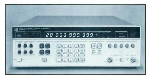
Fig. 1. Model 3325A Synthesizer/ Function Generator produces waveforms with frequencies as low as 1 µHz and as high as 21 MHz for sine waves (to 11 MHz for square waves and 11 kHz for triangles and ramps) with synthesizer accuracy. Output amplitude over the full frequency range is 1 mV to 10 V p-p into 50  $\Omega$  or, with an option, to 40V p-p into 500 Ω over a frequency range of 1 µHz to 1 MHz. All necessary functions can be controlled through the HP interface bus as well as the front panel.
