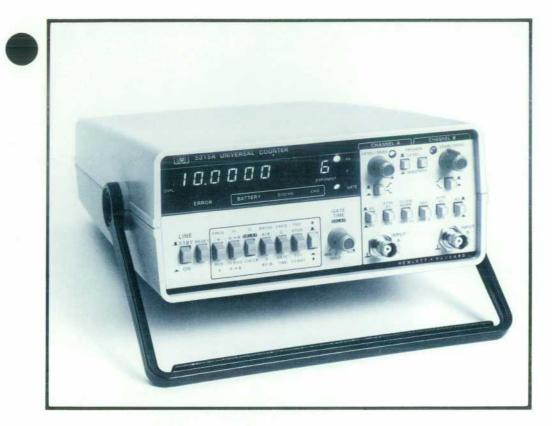
Fig. 1. Model 5315A Universal Counter measures frequency to 100 MHz and time intervals with 100-ns resolution. A reciprocaltaking two-channel instrument with a seven-digit display, it offers mid-range counter performance at a cost much lower than previousgeneration counters. Shown here is the 5315A. The 5315B, the same instrument in a half-rack-width metal cabinet, offers exceptionally low radiated emissions.
