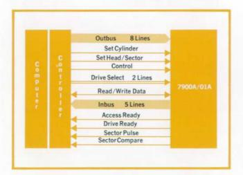
Fig. 1. Interface circuits are partitioned between drive and controller so expensive redundancies are avoided without loss of performance. Bus structure minimizes number of cables.
