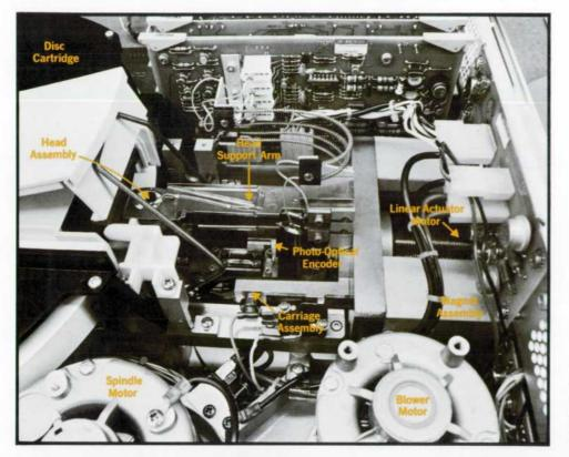
signing the unit for minimum inductance. The coil is wound on a glass-reinforced epoxy tube and permanently bonded to a die-cast aluminum carriage.
