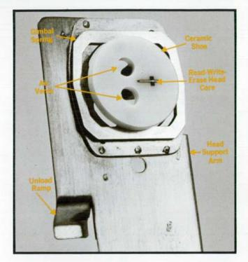
Fig. 3. The HP-developed read/write heads are critical to the drives' ability to operate between 10°C and 40°C. Inhouse production assures control of their characteristics.
