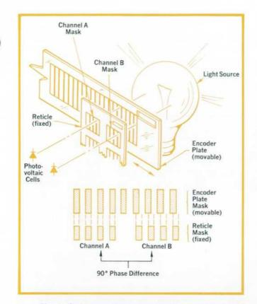
Fig. 3. Optical encoder senses location and direction of read/write heads. Head position and destination are both available in registers at all times.
