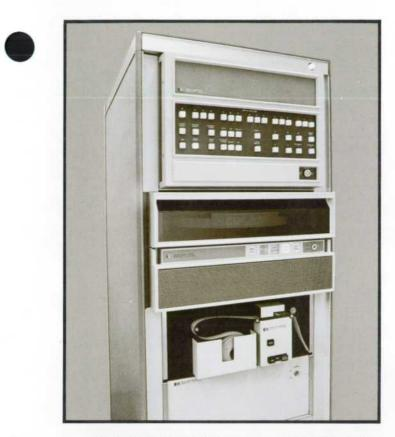
Fig. 1. Model 7900A Disc Drive operates in environments too severe for other drives. It's also fast for a small movinghead drive: average seek time is 30 ms, average latency is 12.5 ms. Data transfer rate is 312,000 bytes per second. Capacity on one fixed disc and one removable cartridge is 5 million 8-bit bytes.
