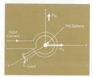
(1) Tuned bandpass filter consists of YIG sphere at center of two mutually orthogonal loops.
