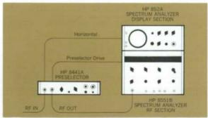
Fig. 2. New HP Model 8441A Preselector, connected to spectrum analyzer as shown, confines displayed signals to a selected frequency range. The preselector is a narrowband YIG filter which automatically tracks a selected harmonic mixing mode of the analyzer's LO and mixer.
