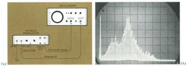
Fig. 6. (a) HP Model 8441A Preselector, with detector and oscilloscope, forms a lowsensitivity but very wideband spectrum analyzer. (b) Spectrum of high-power frequency comb obtained with spectrum analyzer setup (a). Sweep limits are 2 and 12 GHz.
