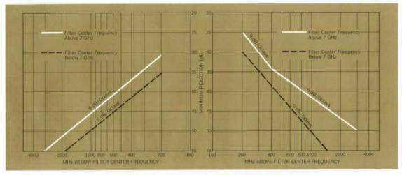
Fig. 5. Selectivity characteristic of Model 8441A Preselector.
