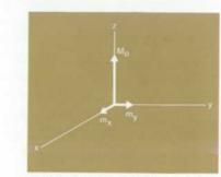
(e) Equivalent representation of precessing magnetization vector.
