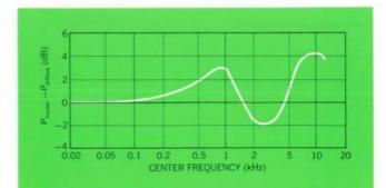
Fig. 2. Difference between equal-loudness-level contours in frontal diffuse sound fields, according to ISO R 454.
