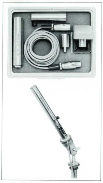
Fig. 3. Loudness analyzer microphone consists of 1" condenser microphone cartridge and preamplifier. Response is flat within  $\pm 1$  dB from 30 Hz to 8 kHz and within  $\pm 2$  dB from 8 kHz to 18 kHz.
