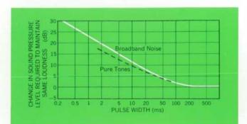
Fig. 7. As duration (pulse width) of a sound decreases, its sound pressure level must increase to maintain same loudness.
