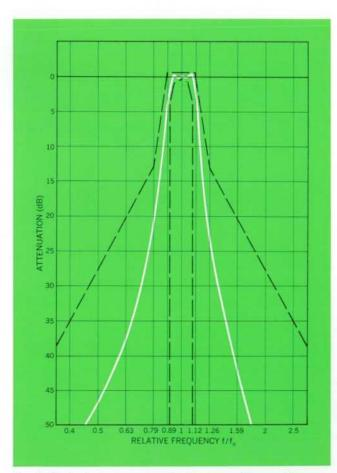
Fig. 6. Typical response curve for ½-octave filter used in loudness analyzer. Response is down more than 20 dB at center frequency of following filter, and down 60 dB at twice the center frequency. Dashed curves show tolerances allowed by international standards.
