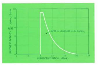
Fig. 7. Masking curve for 1 kHz tone. This is Zwicker's approximation to the way in which a pure tone or narrowband sound (centered at 1 kHz, in this case) excites nerves in the ear corresponding to many frequencies. Masking occurs if the curves corresponding to two or more sounds overlap. Loudness analyzer simulates masking effect by means of a capacitor-discharge circuit which follows tail of curve.
