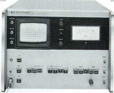
Fig. 1. New HP Model 8051A Loudness Analyzer measures loudness of narrow-band or wideband, continuous or impulsive sounds. Analyzer makes Zwicker-type analysis, gives results which agree well with subjective sensation of loudness. CRT shows loudness density versus subjective pitch; meter shows total loudness.
