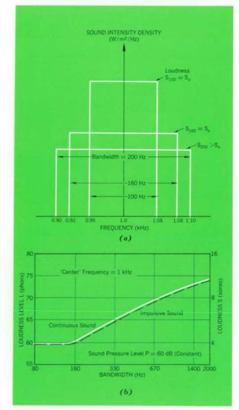
(b) As bandwidth increases, keeping sound pressure level constant as in (a), loudness level is not affected until bandwidth exceeds a critical value. Different center frequencies have different critical bandwidths. At 1 kHz, critical bandwidth is 160 Hz.
