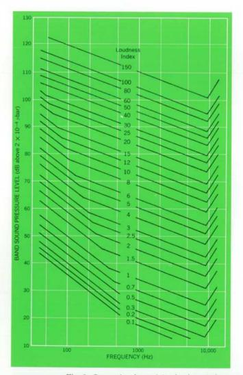
Fig. 9. Curves for determining loudness indexes used in Stevens' method of calculating loudness.
