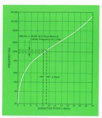
Fig. 4. Subjective pitch scale is different from frequency scale; in subjective pitch, half way between 0 and 4 kHz is about 1 kHz, not 2 kHz. For some as-yet-unkown reason, critical bandwidths at all center frequencies correspond to subjective pitch intervals of the same width. This width is defined as one Bark. (Critical bands are defined in Fig. 3.)
