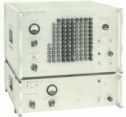
Fig. 1. Pushbutton bank on the HP Model 5105A Frequency Synthesizer permits selection of high-quality signals up to 500 MHz in steps as fine as 0.1 Hz increments.
