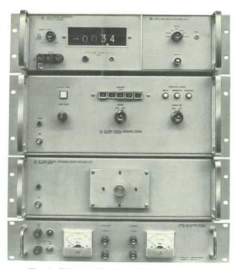
Fig. 1. This complete thermal resistance measurement system speeds evaluation of diodes. In production, it allows fast checking for packaging faults. The diode under test is placed in the heat sink located in the center of the rack second from the bottom.
