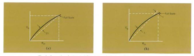
Fig. 3. Comparing the 'terminal linearity' method of specifying gain accuracy (a) with the 'best straight line' method (b) shows that while the 'best straight line' method results in better numbers on specifications, the 'terminal linearity' method results in a more accurate statement of real usefulness.
