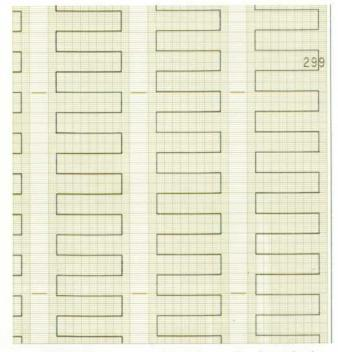
Fig. 4. Chart paper used for ink recording has eight channels, each 4 cm wide with 50 divisions. Recorded square wave shows how ink-pressure modulation prevents loss of trace for stcp-function inputs.
