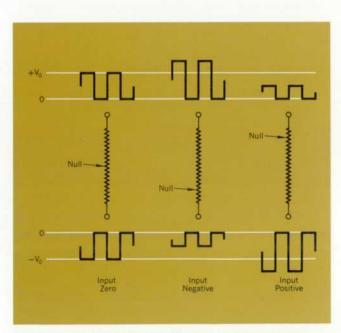
Fig. 8. 20 kHz square waves, 180° out of phase, are applied to ends of transducer resistor, creating a null which is shifted as a function of the input signal. Servo system senses pen position relative to the null and drives pen to follow null.
