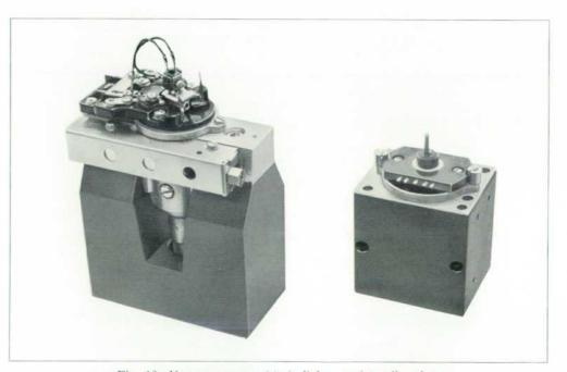
Fig. 10. New pen motor (r), is lighter and smaller than older type (l), and has smaller stray external magnetic field.
