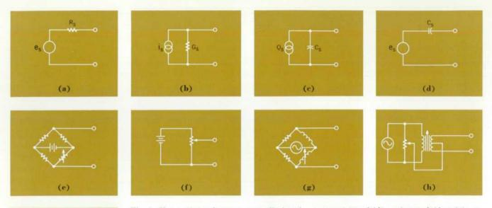
Fig. 1. Classes of signal sources generally found in use with data amplifiers include voltage sources (a), current sources (b), as charge
