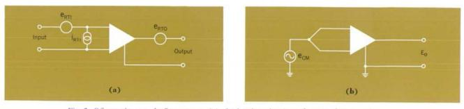
Fig. 2. Offset voltage and offset current (a), both referred-to-input because they are gaindependent, and the voltage referred-to-output which is not gain-dependent, are the major parameters in determining total offset. Insufficient common-mode-rejection is another source of offset error (b). The common mode signal at the output is equal to  $e_{CM}\left(\frac{Gain}{CMR}\right)$ .
