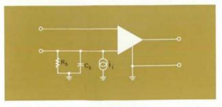
Fig. 4. Sources of additional offset error are due to injected current, i<sub>1</sub>, source resistance and capacitance.
