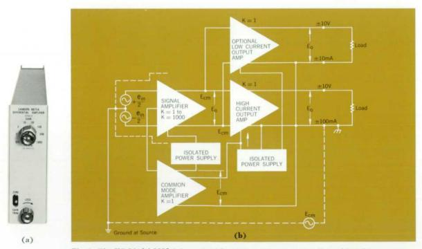
Fig. 3. The HP Model 8875A Data Amplifier (a) uses a common mode amplifier (b) to provide good common mode rejection wthout the use of a specially shielded power transformer.
