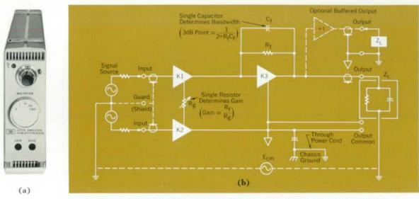
Fig. 2. The new HP Model 2470A Data Amplifier (a) is a differential design consisting of three amplifiers, K1, K2 and K3 (b). Amplifiers K1 and K2 are identical. Power supplies for the three amplifiers are completely isolated from each other to preserve the common mode rejection offered by the design.
