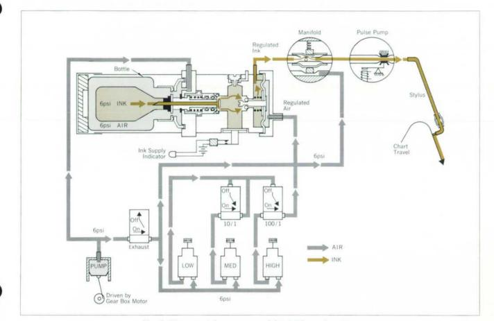
Fig. 5. Diagram of the pressure-modulated ink supply system. One pen is shown, although the manifold supplies all eight.
