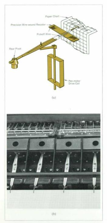
Fig. 6 (a). Pen drive mechanism is simple, yet very linear. As pen motor rotates, pen tip describes a line that is straight within 0.005" across 4 cm channel. Position-sensing transducer is located near pen tip to detect linkage errors. Pickoff wire does not touch wirewound resistor, so transducer wear is not a problem. (b). Transducer resistors can be seen just below transverse rod in photograph.
