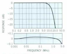
Fig. 3. Basic FLAT frequency response of oscilloscope is down less than 0.1 dB below 4.5 MHz, less than 1 dB at 8 MHz, 3 dB at 10.5 MHz, then has very fast rolloff and is down 20 dB at 20 MHz. This eliminates high-frequency noise if present on incoming line. Lower diagram shows ±0.05 dB flatness below 1 MHz.
