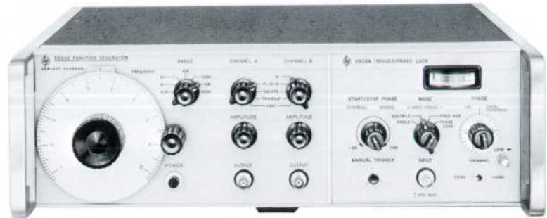
Fig. 3. New -hp- Model 3300A Low Frequency Function Generator, shown here with Trigger/Phase-Lock Plug-in, is voltage-programmable through rear panel connector. Separate outputs supply any two of available waveforms (sine, square, triangle) or may be used together in balanced push-pull configuration.
