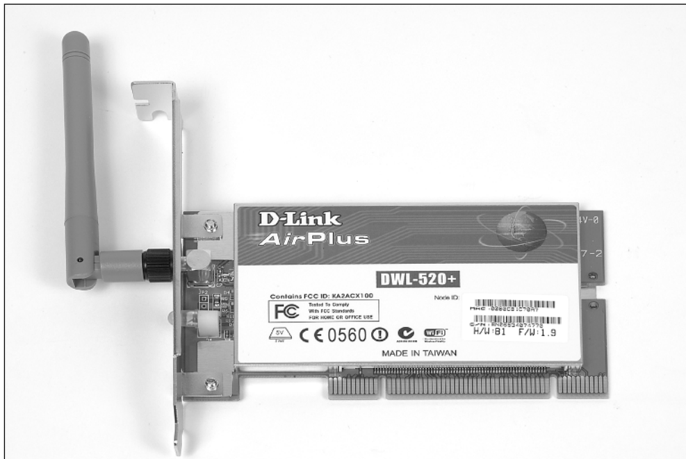
Figure 5-3: This PCI card adds WiFi wireless networking to a desktop PC.
