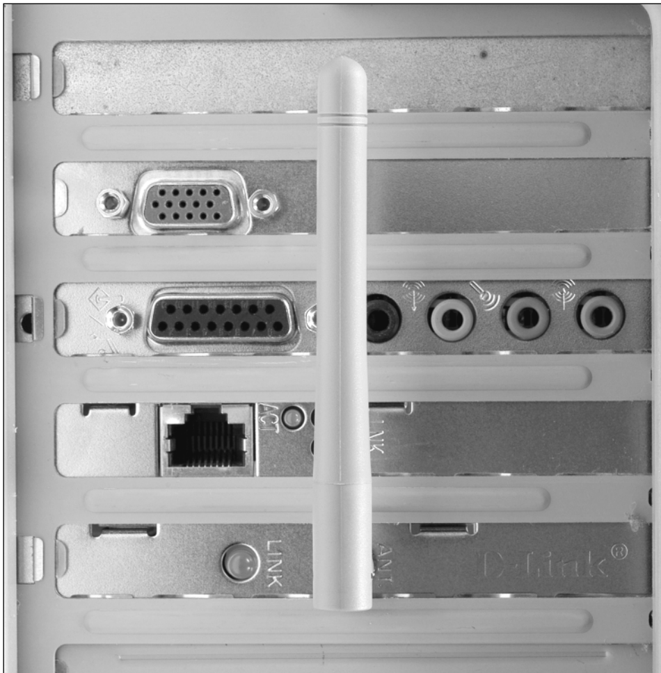
Figure 7-3: The antenna should be vertical to the floor.
