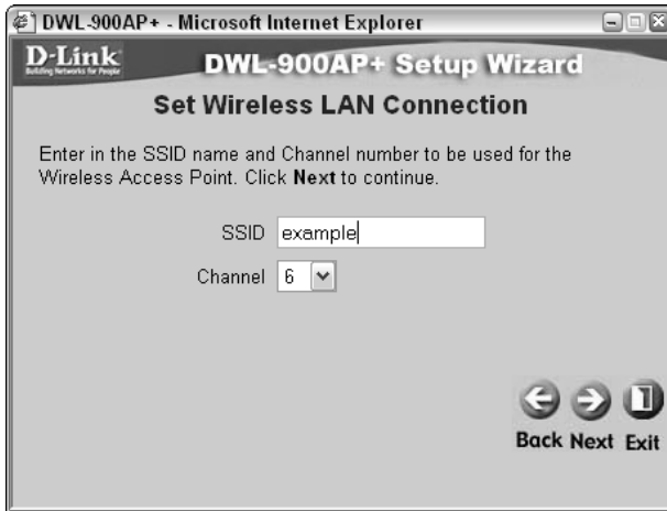
Figure 7-14: This screen lets you select an SSID name and a channel number for your AP.
