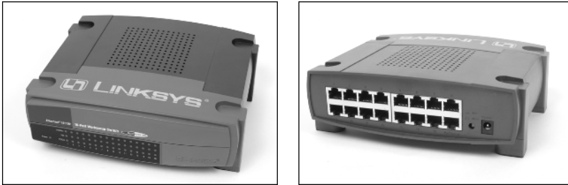
Figure 5-8: This 16-port switch is a little large for most home networks, but it has plenty of room to grow.
