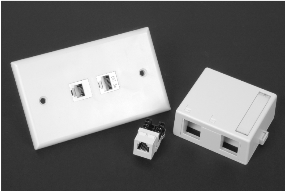
Figure 6-5: A modular wall plate (left) fits into a standard outlet box and holds two jacks for Ethernet, telephone, TV, or speaker cables. The jacks (center) simply snap into the openings on the plate. The surface-mount jack (right) works the same way but can be mounted on any flat surface.
