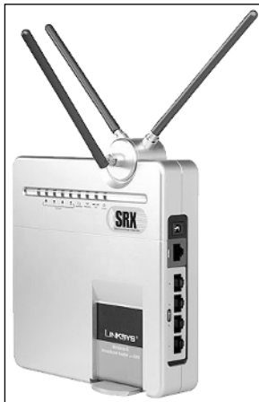
Figure 4-4: The Linksys WRT-54G wireless router uses three antennas for better coverage. (Photo courtesy of Linksys)
