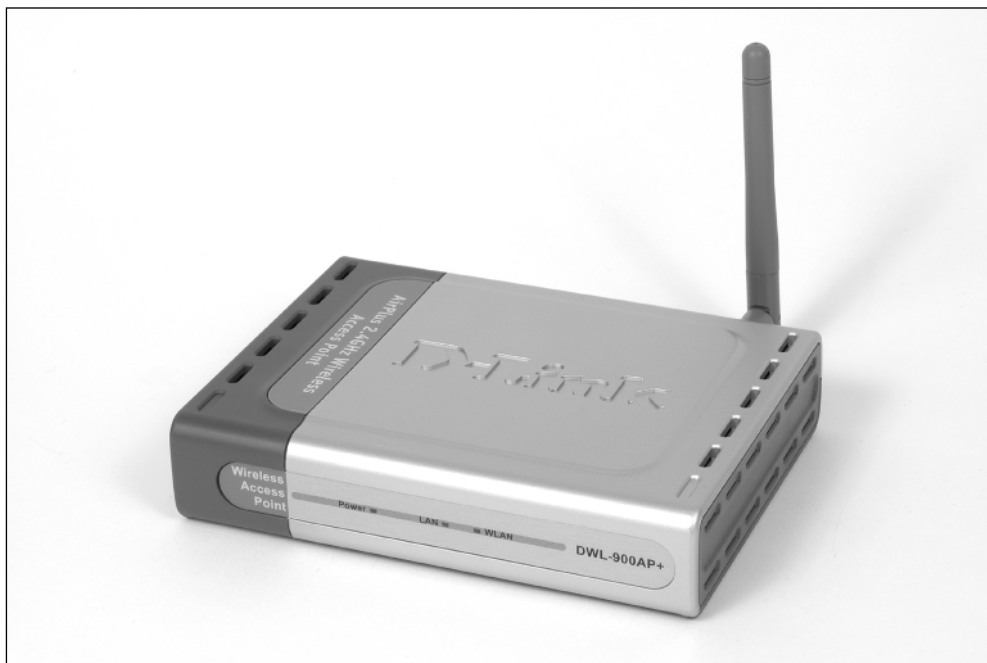
Figure 5-11: This access point is about the size of a paperback book.
