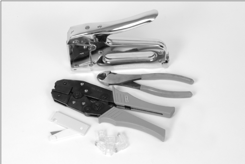
Figure 6-4: These are a few of the tools you'll need for a neat, professional cable installation. They are (from top to bottom) a cable stapler, a wire cutter, an RJ-45 connector crimper, and a cable stripper. You'll also need a supply of RJ-45 connectors.
