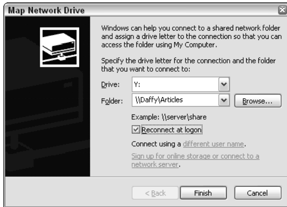
Figure 3-7: You use the Map Network Drive dialog box to create drive mappings.
