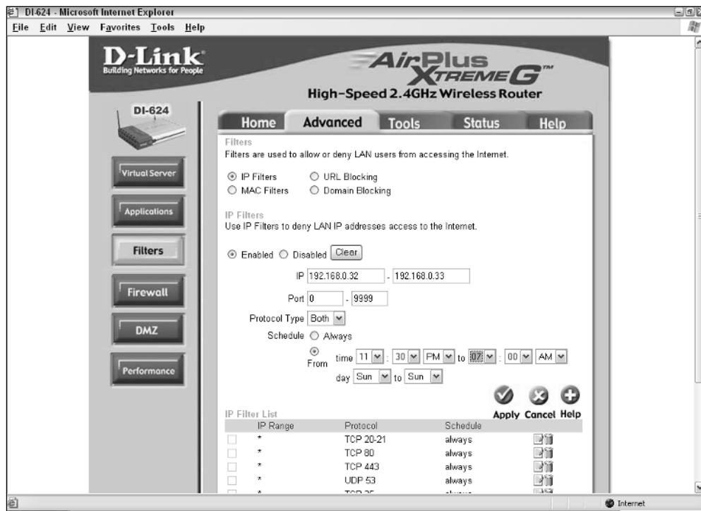
Figure 14-4: This D-Link router lets you enable and disable filters on a scheduled basis.
