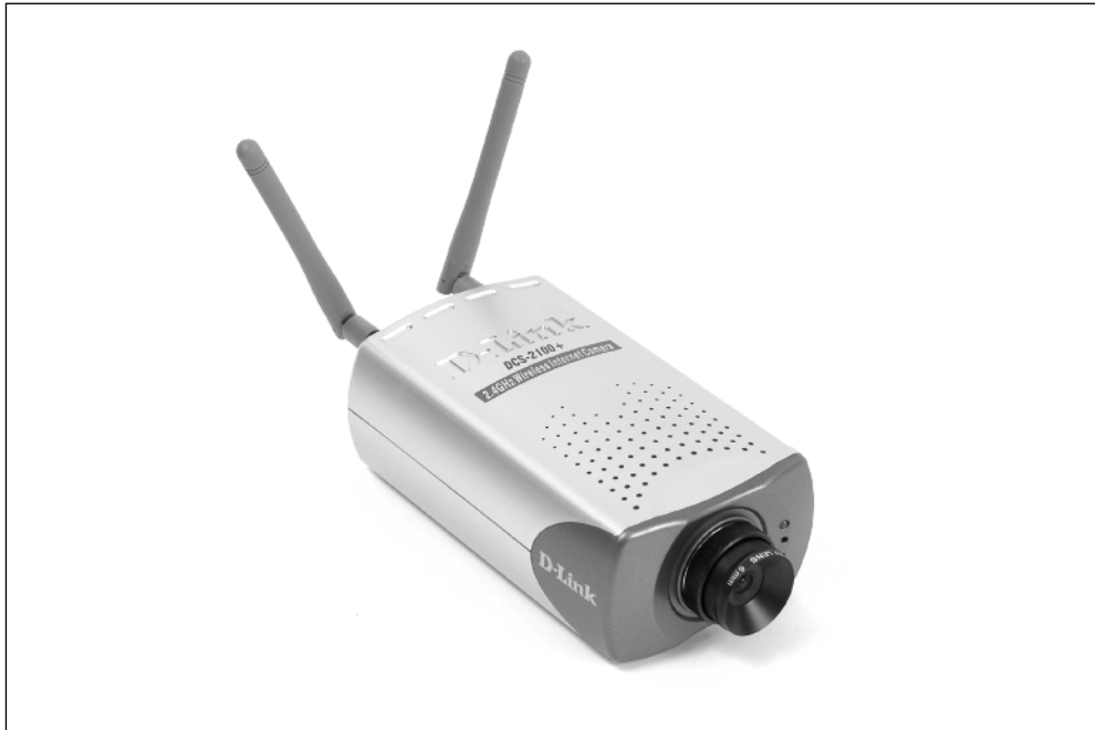
Figure 12-29: The D-Link Wireless Internet camera has a built-in Web server, along with wired Ethernet and WiFi wireless connections.
