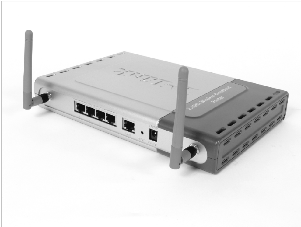
Figure 1-3: D-Link calls its model DI-624 a Wireless Broadband Router. It combines a four-port Ethernet switch, a wireless access point, a router, and a firewall into one compact, inexpensive unit.
