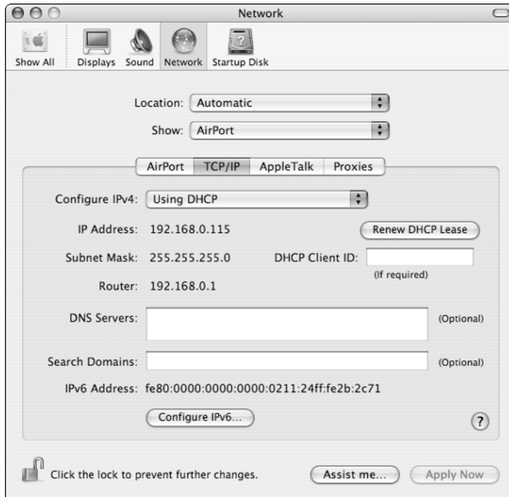
Figure 3-3: The Mac OS/X Network settings control panel allows you to select manual or automatic IP addressing for each network connection. This example shows the IP settings for an AirPort wireless network connection.
