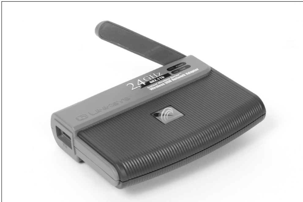
Figure 5-4: This wireless USB adapter comes with a long USB cable, so you can position the adapter for the best signal reception.
