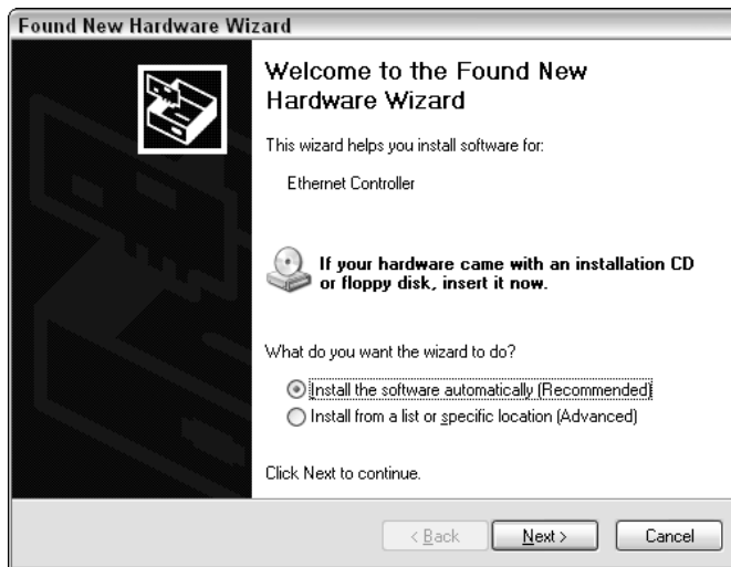
Figure 7-4: The Windows Found New Hardware Wizard appears when you first insert a new adapter card.
