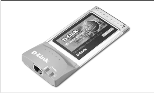
Figure 5-5: This CardBus 10/100 Ethernet card features a built-in Ethernet jack with link and activity indicator lights.
