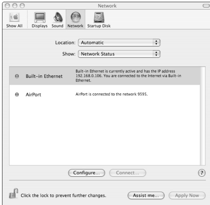
Figure 6-9: The Network dialog box shows the status of your Mac's network connections at a glance. In this example, both the Ethernet and AirPort wireless connections are active.
