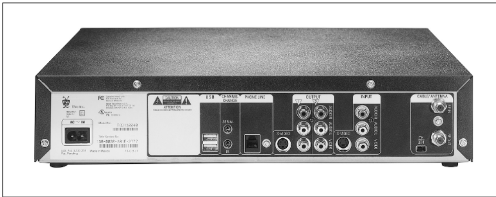
Figure 2-11: The rear panel has connections for your VCR, satellite receiver, cable box, TV set, stereo system, and two USB ports for add-ons like a broadband Internet connection.
