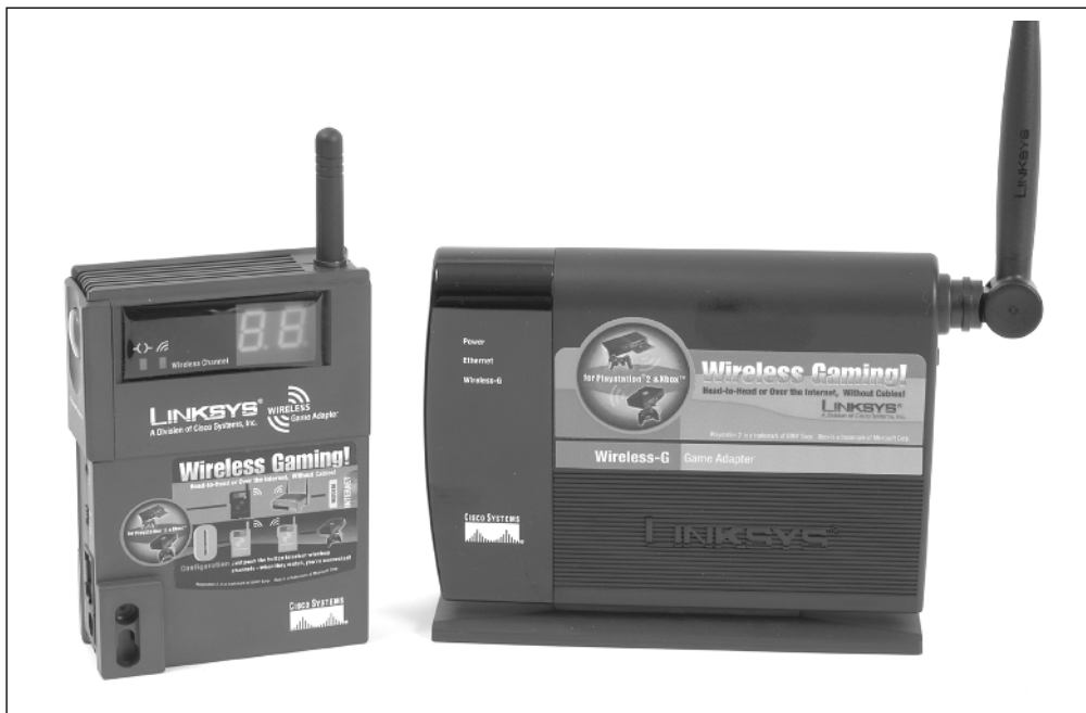
The Linksys Wireless-B (left) and Wireless-G network gaming adapters add wireless connectivity to Ethernet-equipped game consoles.
