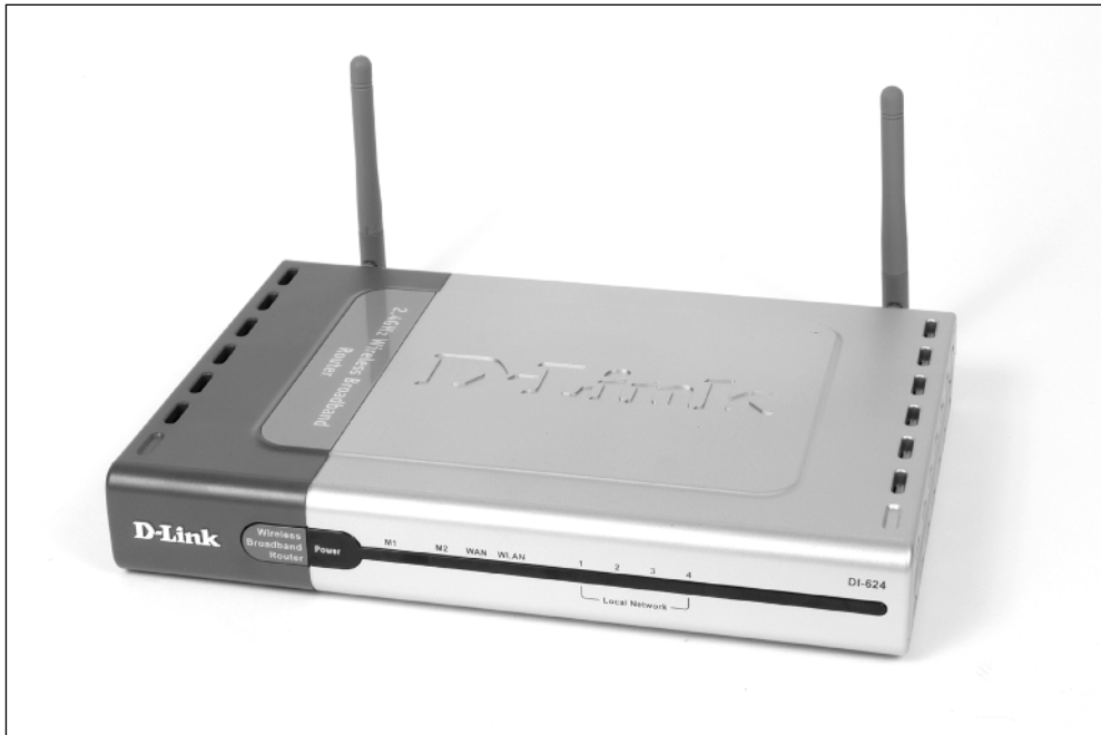
Figure 5-14: This router includes a wireless access point with two antennas as well as a four-port Ethernet switch.
