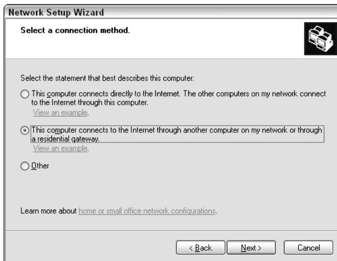
Figure 8-4: You use this step to tell the wizard if this computer will be an ICS server.
