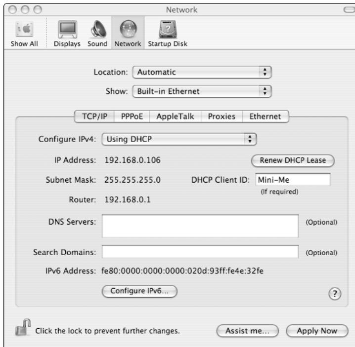
Figure 6-10: The Network dialog allows you to change the settings for your Mac's Ethernet connection. In this example, the Ethernet connection is set for automatic configuration, and you can see the IP address automatically assigned by the router.
