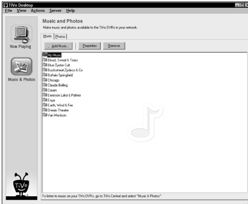
Figure 12-17: The TiVo Desktop lets you choose the files available for playback on the TiVo DVR.
