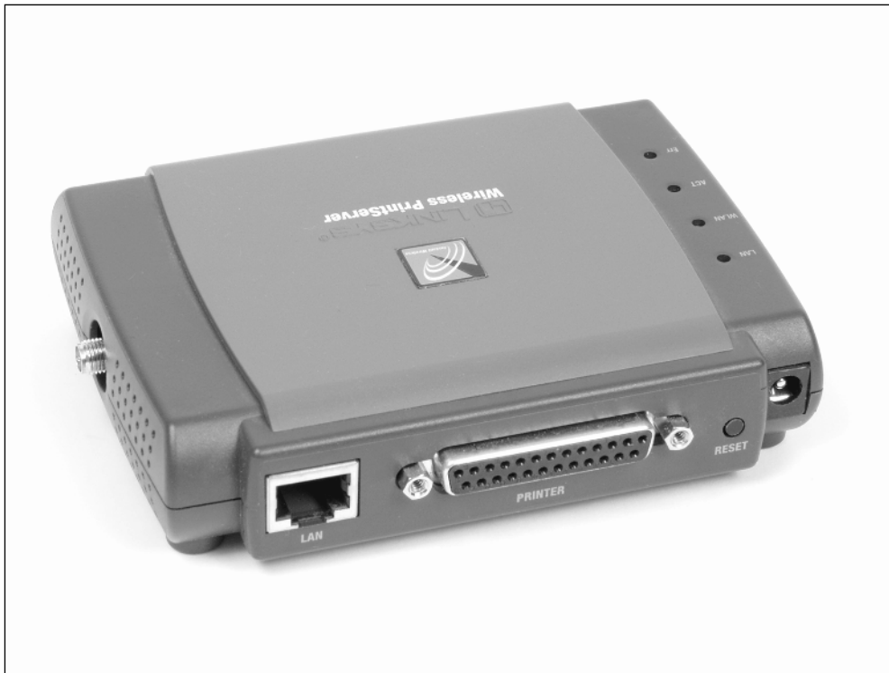
Figure 2-8: This network print server is about the size of a deck of playing cards and operates with wired or wireless networks. The small connector on the left side of the picture is for a wireless antenna; the rear panel provides connections for wired Ethernet (left), a parallel printer (center), and the power cord.
