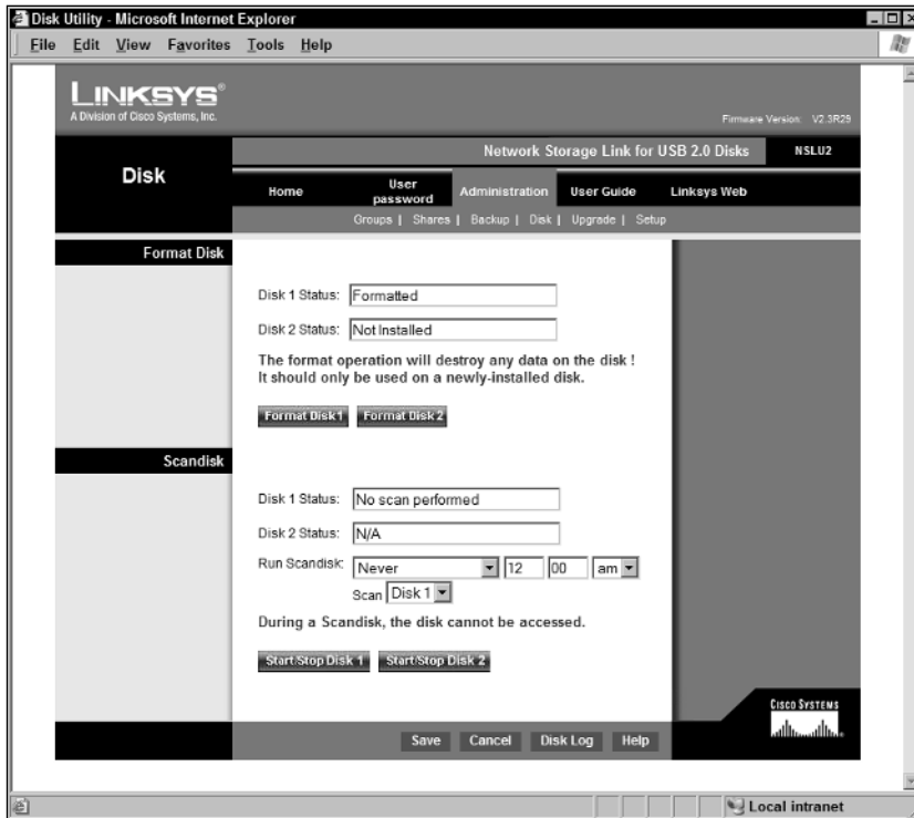
Figure 14-11: The disk status screen shows the operational status of the disk drives attached to the server. Note that in this example, I have already formatted Disk 1.
