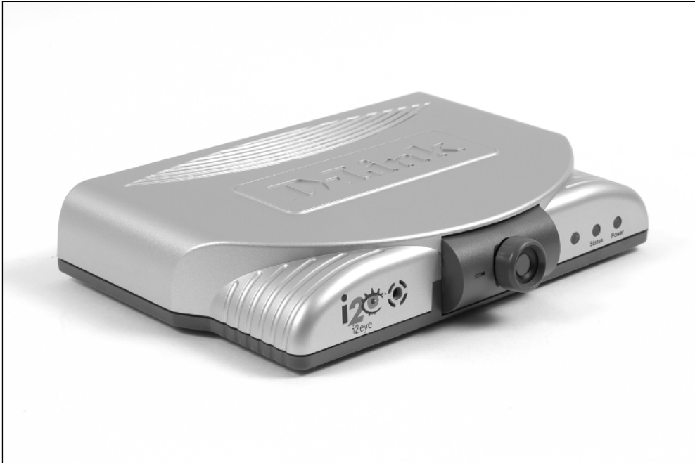
Figure 12-33: The D-Link i2eye sits on top of your TV set. The lens (center) swivels up and down to adjust for the height of your TV screen.
