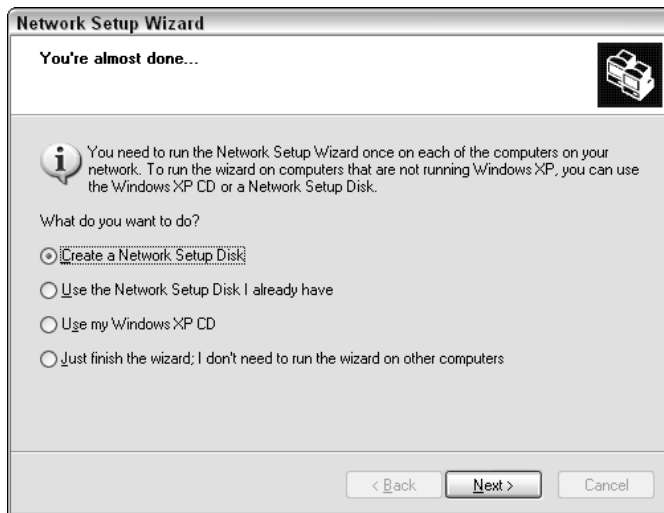
Figure 8-10: You can save the settings from the Network Setup Wizard and use them on another computer.
