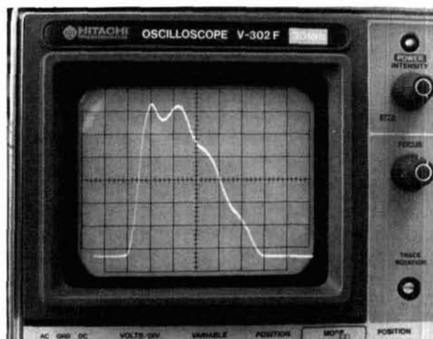
fig. 7E. Crystal filter load impedance is too low, resulting in a noticeable loss of audio frequency response and confusion in setting the BFO frequency.
