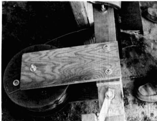
fig. 3. Wire is fed from mounted spool through guide tube into trench.
