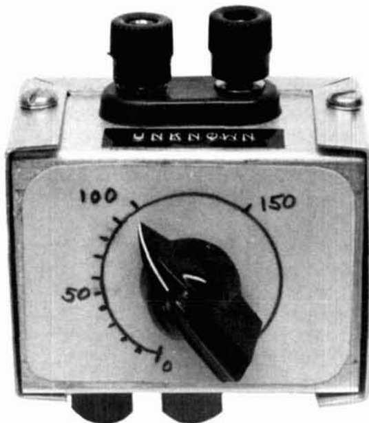
fig. 4. Panel view of the RF bridge shows the calibration of the variable (balance) resistor. This is done using an ohmmeter — no trick to it all! Make sure the variable resistor value increases in a clockwise direction.
