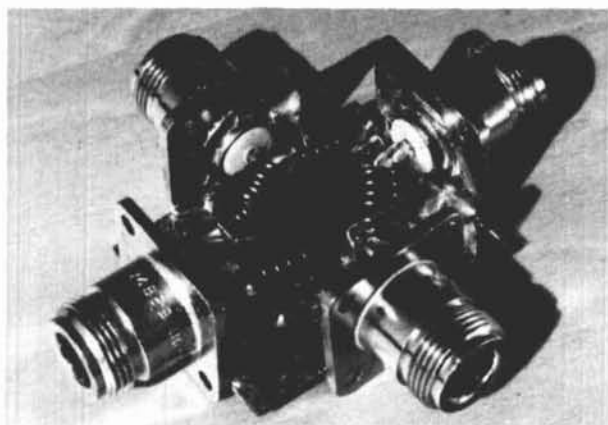
At frequencies below 30 MHz, lumped constants offer less loss than coaxial cable to form compact hybrids.
