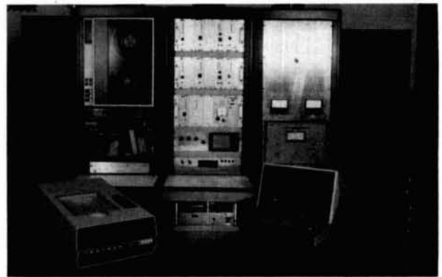
fig. 2. One of the few digital ionosondes in the world, this system developed by the Space Environment Laboratory provides new capabilities — within a single system — to determine ionospheric structure and magneto-ionic effects in general.
