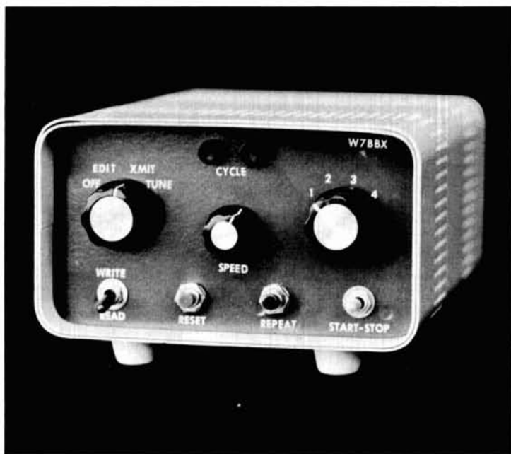
Front panel of programmable contest keyer. Set and forget controls, and input and output jacks, are on rear panel.
