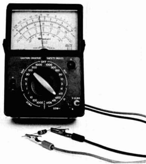
fig. 3. The meter pointer should rest somewhere near midscale for best accuracy when making resistance measurements. This can be accomplished with the "range" switch which is calibrated in decade increments.
