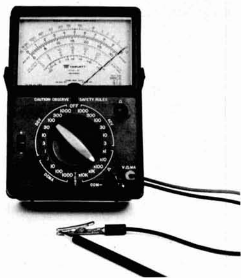
fig. 2. The needle should move up scale to the zero ohms mark when the test leads are shorted together. If the needle doesn't align with the zero ohms mark, adjust the "ohms" or "zero ohms" control on the front of the instrument.
