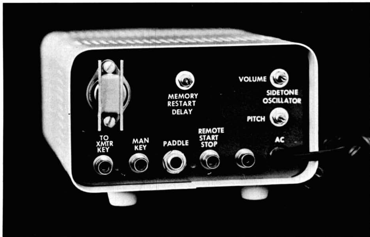
Controls and receptacles on rear panel. Although not labelled, one jack is for grid-block keying; the jack labelled "to xmtr key" is for cathode-keyed transmitters.
