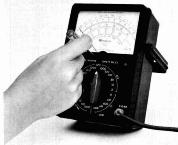
fig. 1. Before making any resistance or voltage measurements, make sure the meter needle is zeroed. If it's not, adjust the mechanical zeroing screw just below the meter face on the front of the vom. This adjustment shouldn't be required very often, but you should always check the mechanical zeroing before you use the instrument.
