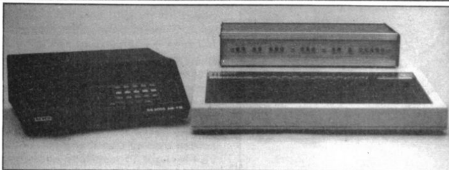
The necessary 'in door' equipment — the AR4200 receiver, a BBC 'B' micro and the interface.
