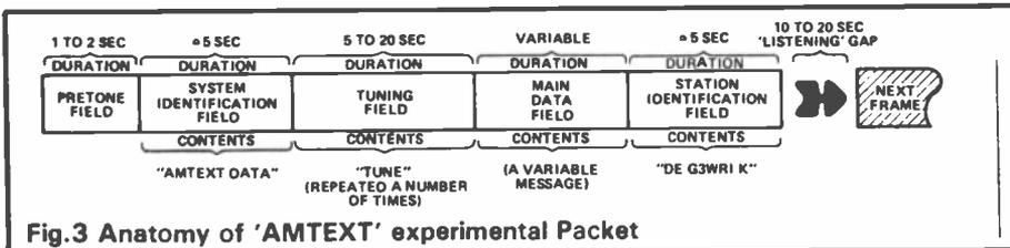
Fig.3 Anatomy of 'AMTEXT' experimental Packet
