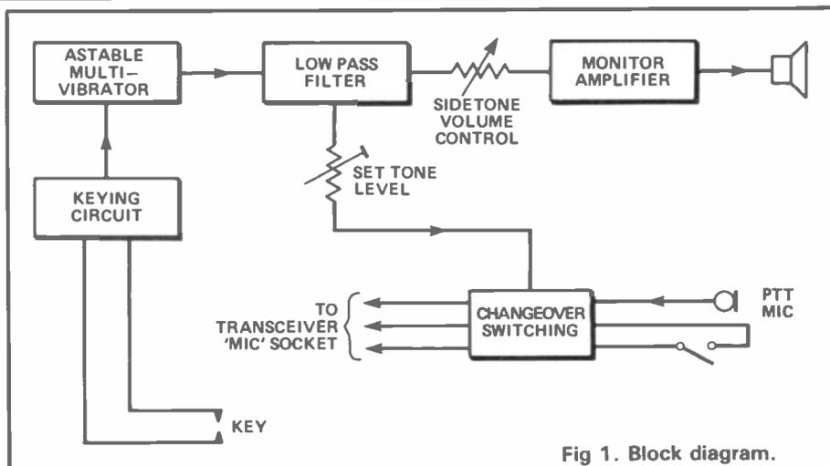
Fig 1. Block diagram.
