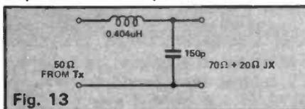
capacitor a small degree of adjustment can be made. These units are very simple to make and it is an easy job to make one up for each band you wish your piece of 'wet string' on. These may be simply swapped over when changing bands, safe in the knowledge that on each of these, your antenna is
