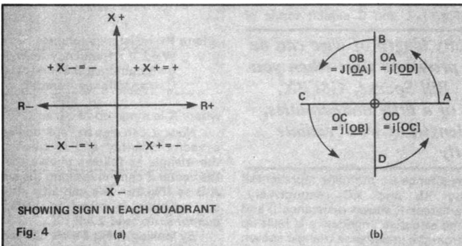
values of SWR will show the variation in the  $Z = R \pm$  vector equation. Without going into details, the technique involved was to measure the SWR at the transmitter end of the aerial feeder cable, then insert a 27 ohm resistor in series with the coax inner and repeat the measurement. (*This process is not to be recommended with a Solid State PAI - Ed.*) It was then possible to determine the R and X values by Smith Chart Analysis (more of this later). These are given in Table 1.
