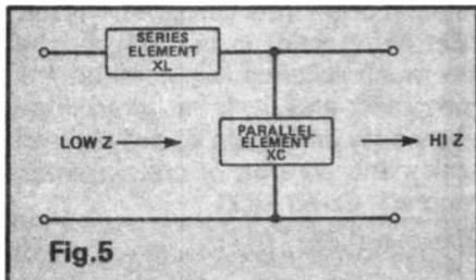
The simple L network shown nearby in Fig.5 will transform a low impedance to a high impedance if connected as shown. By reversing the input and output a high impedance will finish as a low impedance. The observant reader will spot something straight away (See Fig.6 for an extra hint).
