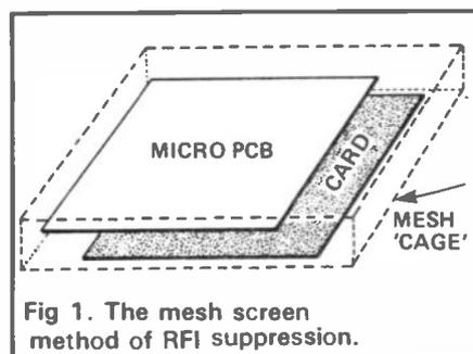
Fig 1. The mesh screen method of RFI suppression.
