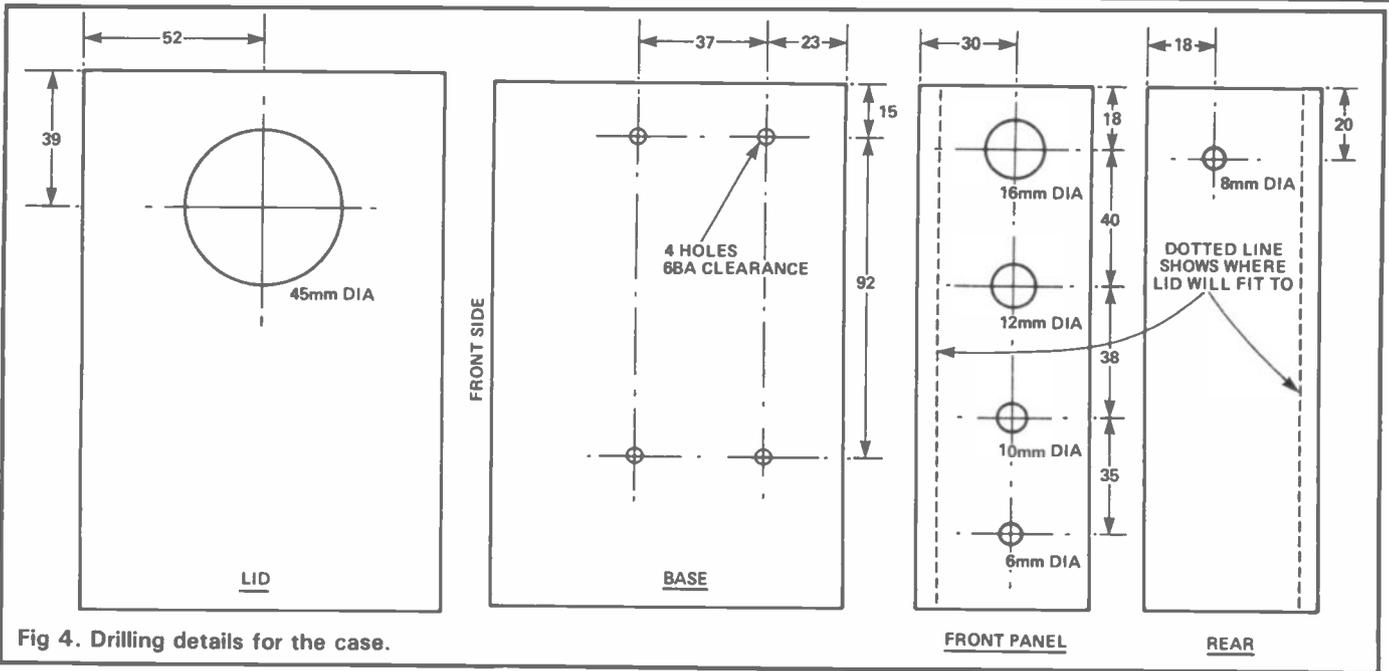
Fig 4. Drilling details for the case.
