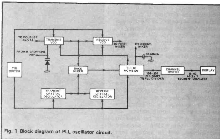
Fig. 1 Block diagram of PLL oscillator circuit.
