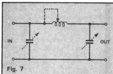
The idea is to transform the typically high output impedance of the valve down to about 25 ohms and then step it up to between 25 and 500 by making the capacitors variable and the coil tapped. The centre transformation point varies along the coil with frequency and finds its own balance point. The value it transforms down to in the centre of the coil is about 25 ohms. Look further into this arrange-
