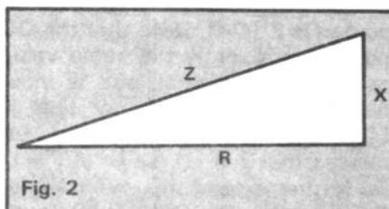
This can be reduced to  $Z = \sqrt{R^2 + X^2}$ . If we think back to our basic tuned circuit theory,  $X = X_L - X_C$ . At resonance  $Z = R$ , the resistance of the tuned circuit, because  $X_L$ , the inductive reactance of the tuned circuit, is equalled and cancelled out by  $X_C$ , the capacitive reactance of the circuit.
