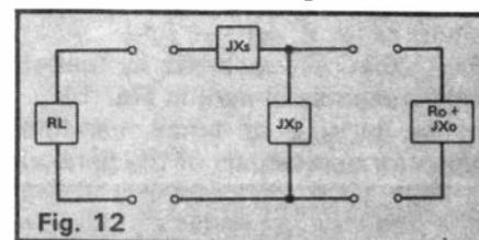
Taking as an example, an aerial on 20 metres was found to have an SWR of 1.6 normal and 1.9 with the resistor in series. This showed 70 ohm + j20 ohm
