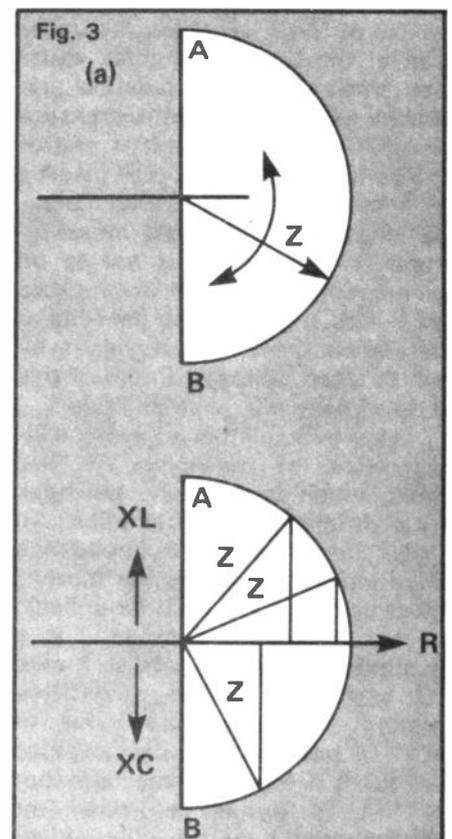
that, for any value of Z there is a large variety of values of R and X which can give Z. Unfortunately, this means practically that a simple impedance bridge connected between our aerial and low power transmitter will be able to give the value of Z but *not* those of X and R. X and R can have *any* value within the limits shown by the arc of the circle.
