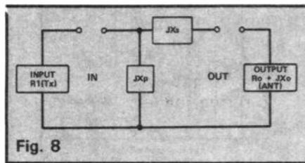
we have the above (Fig.8). The transmitter output is resistive. The series element has reactance, the parallel element has reactance, the load has resistance and reactance. We can now derive the following:-
