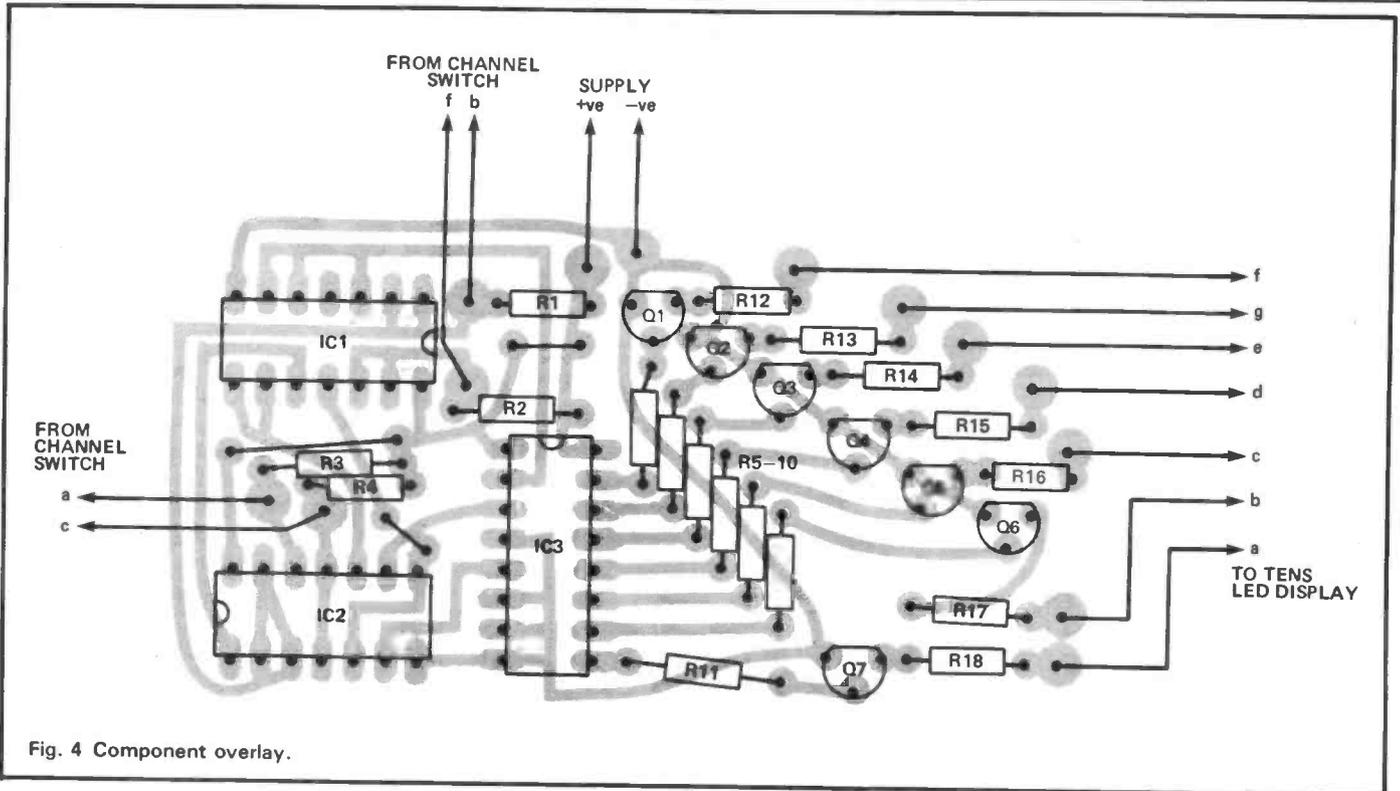
Fig. 4 Component overlay.
