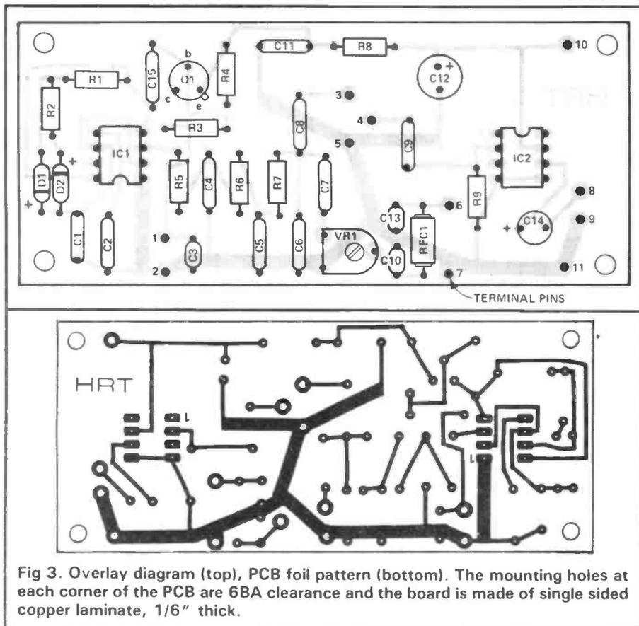
Fig 3. Overlay diagram (top), PCB foil pattern (bottom). The mounting holes at each corner of the PCB are 6BA clearance and the board is made of single sided copper laminate, 1/6" thick.
