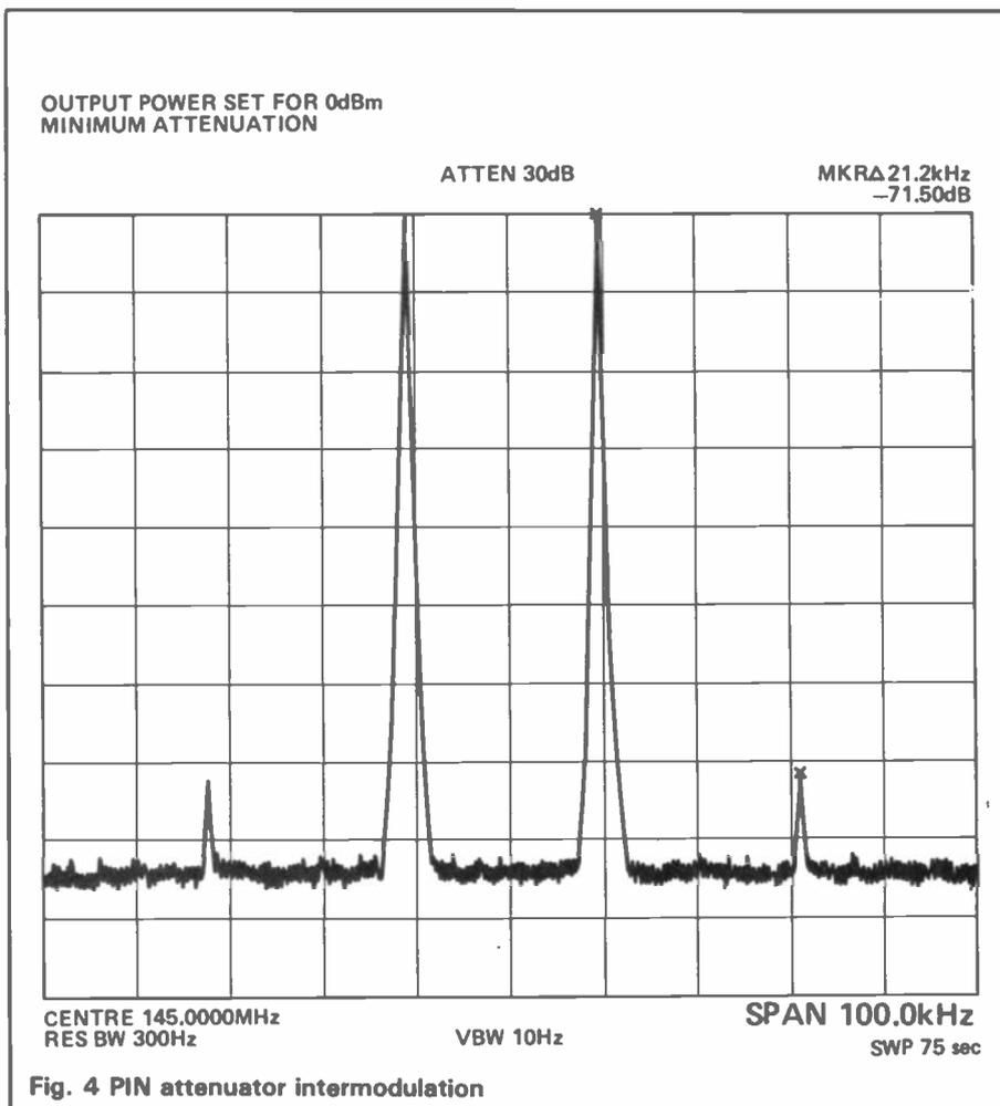
Fig. 4 PIN attenuator intermodulation
