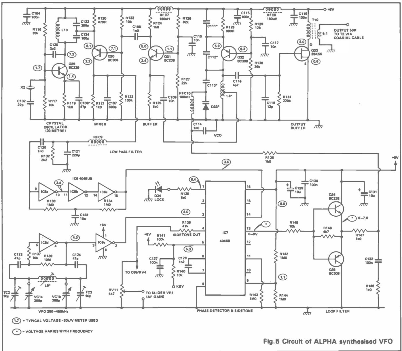
Fig.5 Circuit of ALPHA synthesised VFO
