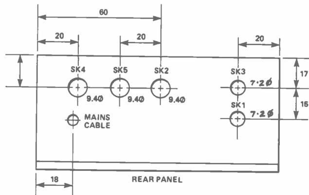
Fig. 6 Enclosure suitable for both 2m control units
