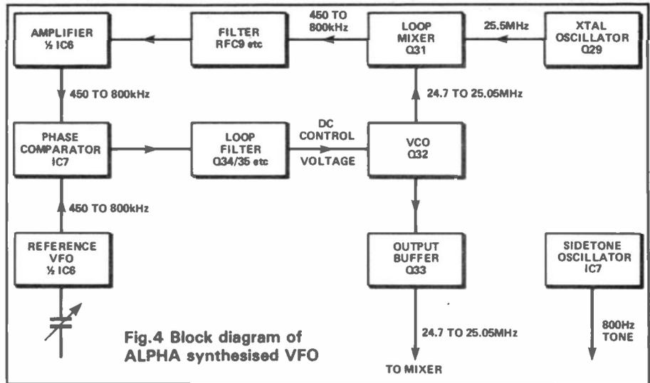
Fig.4 Block diagram of ALPHA synthesised VFO
