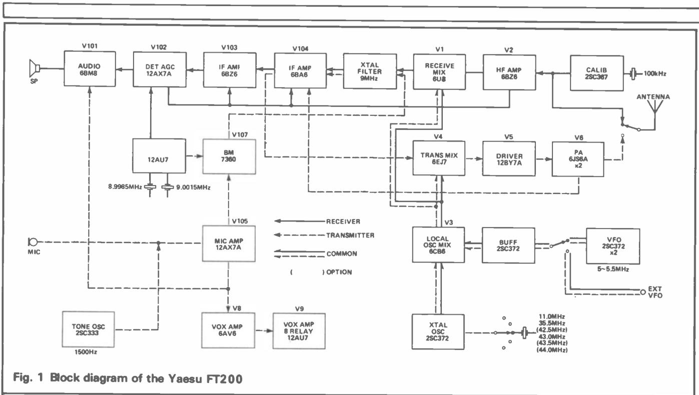
Fig. 1 Block diagram of the Yaesu FT200
