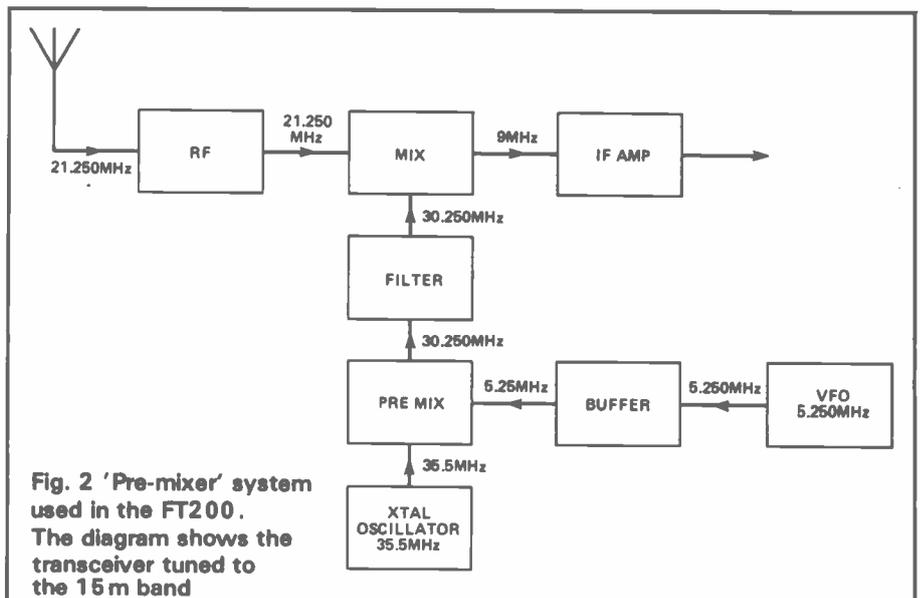
Fig. 2 'Pre-mixer' system used in the FT200. The diagram shows the transceiver tuned to the 15m band
