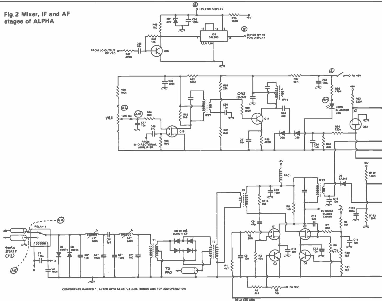
type of circuit, it is essential that frequencies outside the communications speech band are removed before application to the limiter. This filter function is provided by the second order filter ahead of the clipper, Q21. RV3 sets the level of processed audio going to the IC balanced mixer, IC3.
