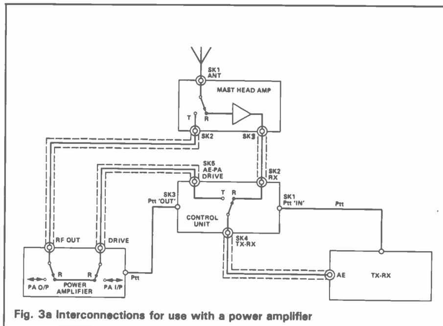
Fig. 3a Interconnections for use with a power amplifier
