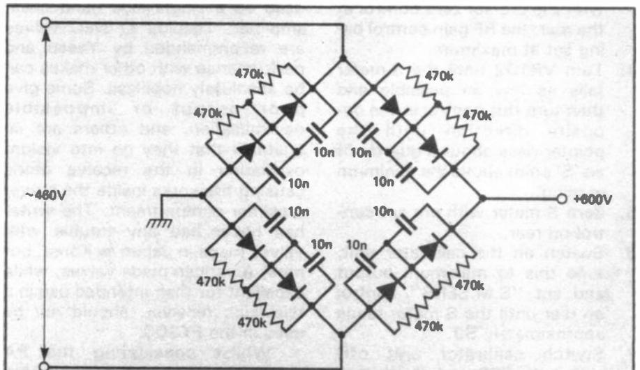
Fig. 3 In the event of trouble with the HT rectifiers, not uncommon with the FT200, they should be replaced by a bridge of 8 BY127 rectifiers as above
