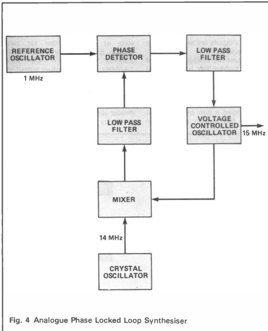
Fig. 4 Analogue Phase Locked Loop Synthesiser
