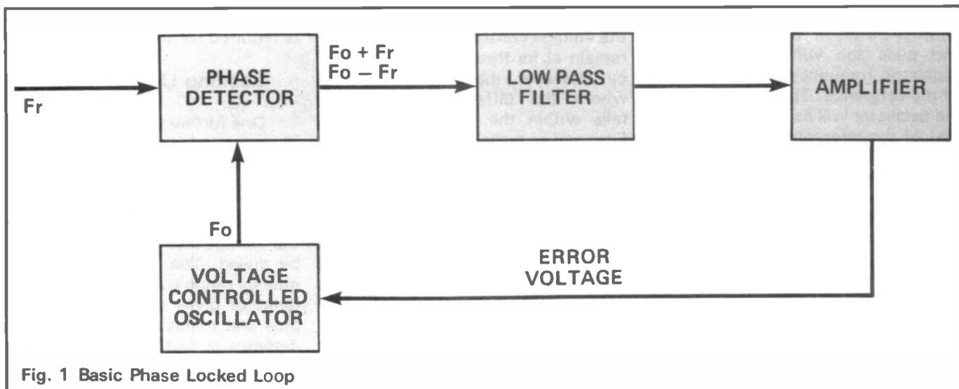
Fig. 1 Basic Phase Locked Loop
