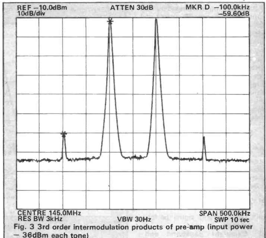
Fig. 3 3rd order intermodulation products of pre-amp (input power - 36dBm each tone)
