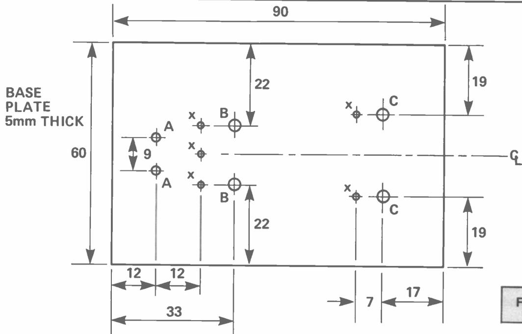
HOLES A = 6BA tapped (or clear) to fix 3 way connector block
