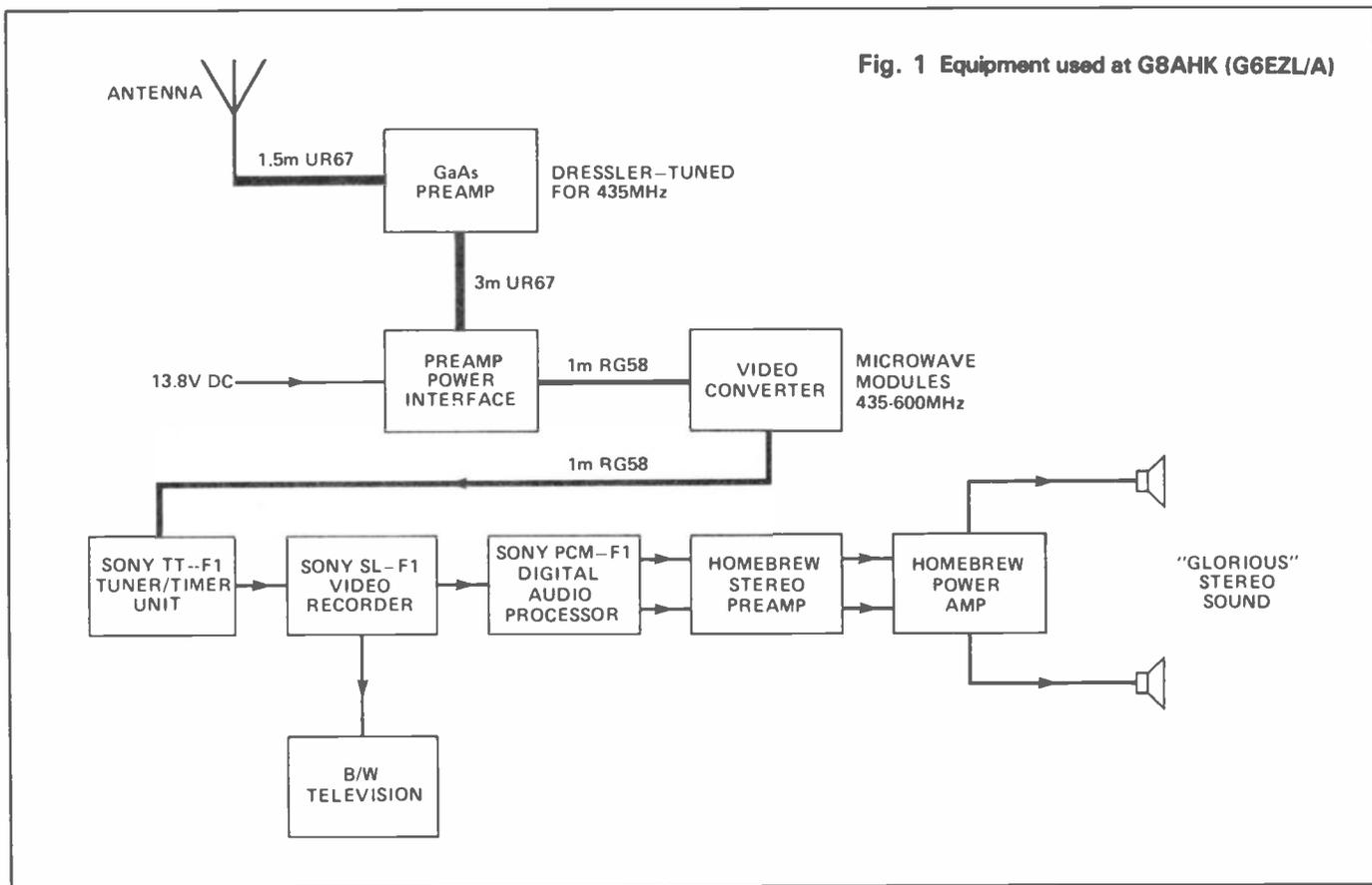
Fig. 1 Equipment used at G8AHK (G6EZL/A)
