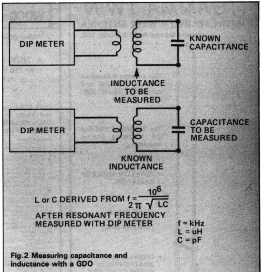
tinuity for coupling into. A better way is to use an *external coupling loop* to the dip meter — actually parting the winding will change the resonant frequency anyway as you will be changing the distributed capacitance around the winding.
