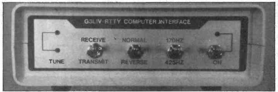
Fig.7. The ready-made unit that is self-contained and derives power from the computer.
