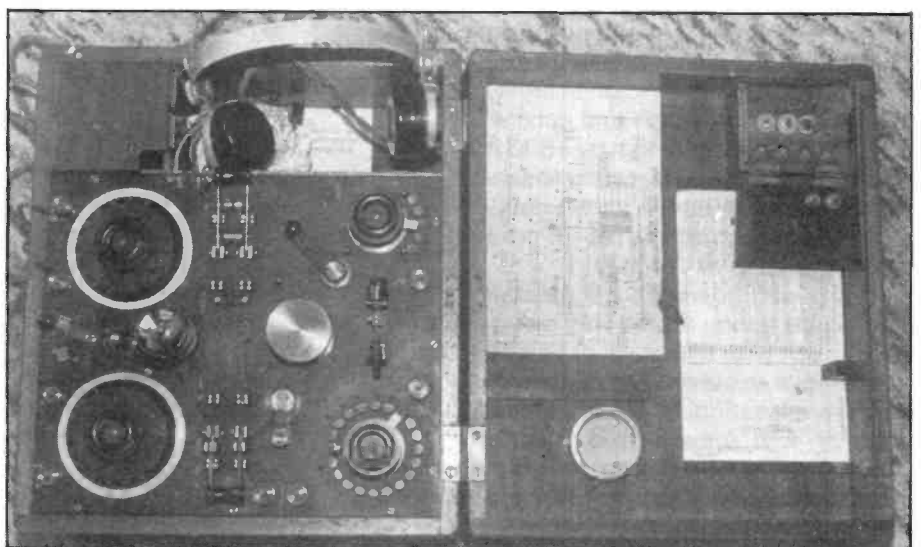
Spark Tx and Rx used by G6GR and his father for their first amateur contacts in 1922.
