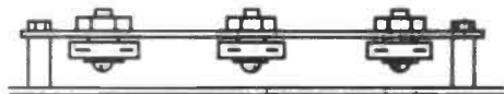
Fig. 2 The Multiplexer is ideally contained in a diecast box 17 x 12 x 5 cm with the circuit constructed on the underside of the box lid. Lower illustration shows mounting for C5, 6 and 7.
