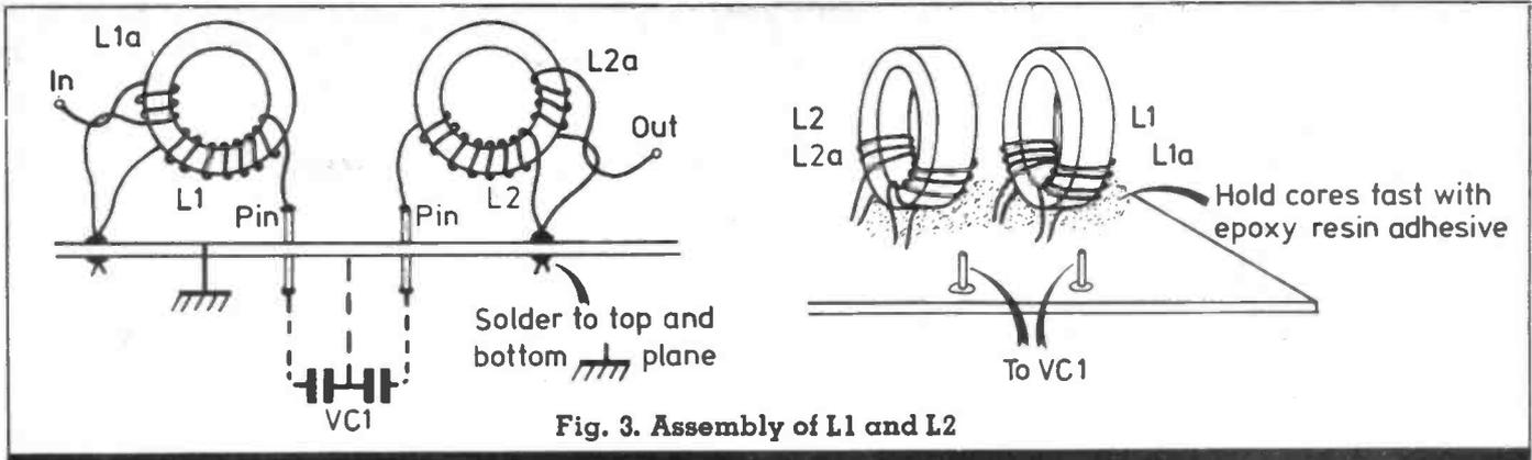
Fig. 3. Assembly of L1 and L2
