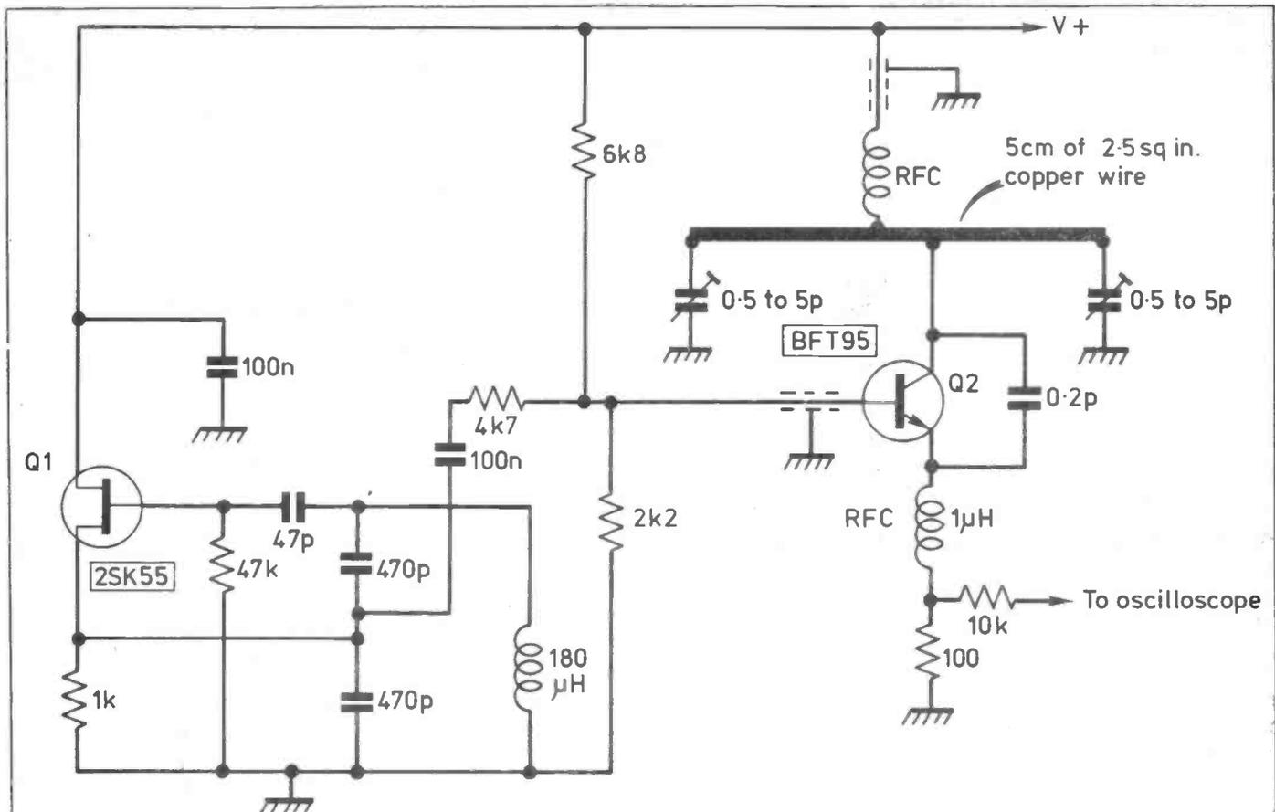
Fig. 5. 23cm Super regenerative test circuit.
