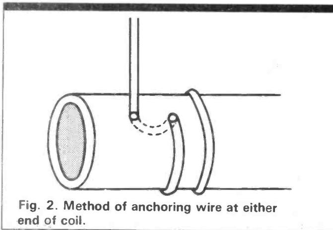
Fig. 2. Method of anchoring wire at either end of coil.
