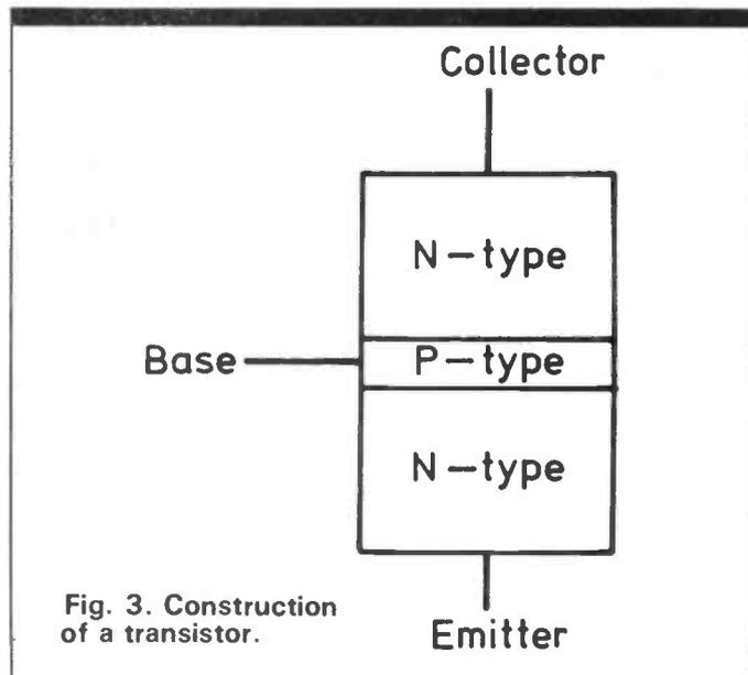
Fig. 3. Construction of a transistor.
