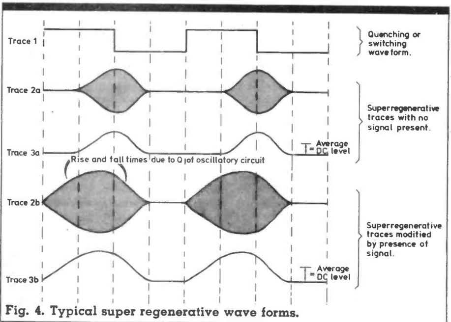
**Fig. 4. Typical super regenerative wave forms.**
