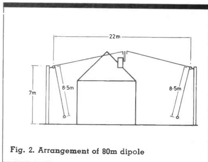
Fig. 2. Arrangement of 80m dipole
