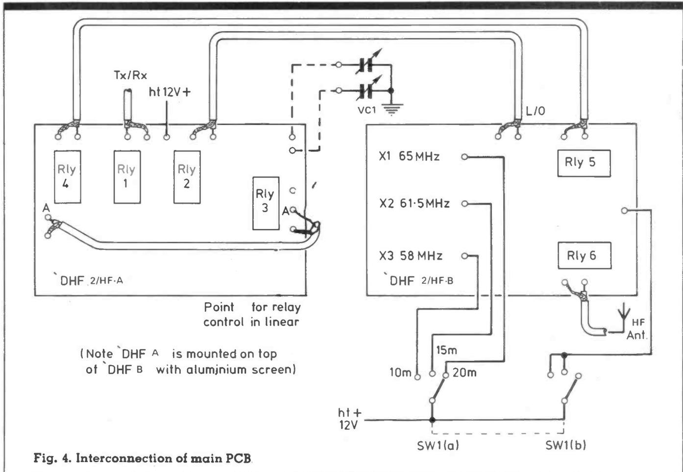
Fig. 4. Interconnection of main PCB
