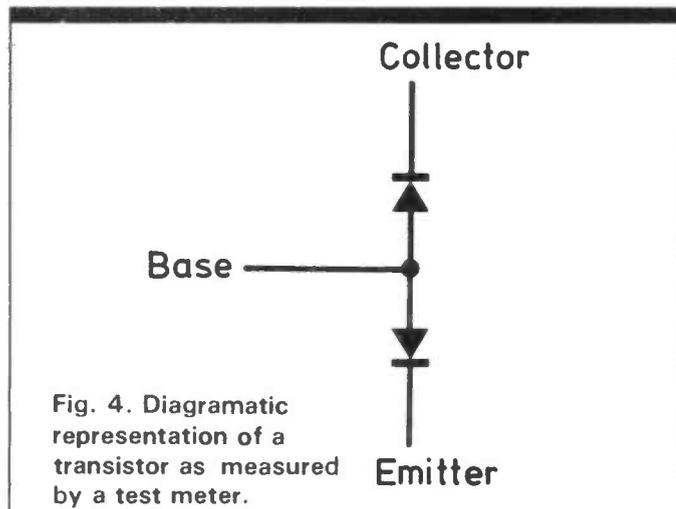
Fig. 4. Diagrammatic representation of a transistor as measured by a test meter.
