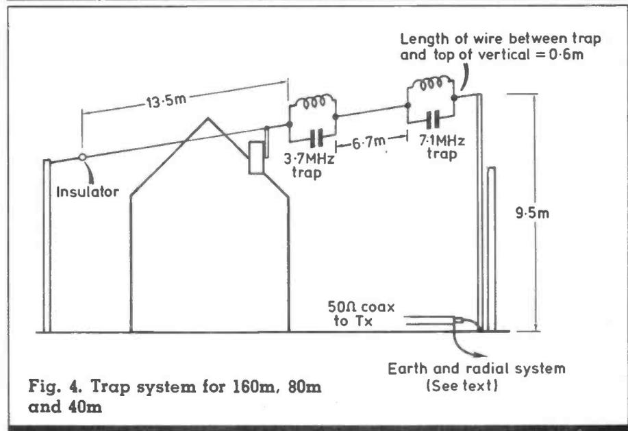
Fig. 4. Trap system for 160m, 80m and 40m
