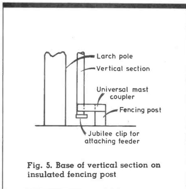
Fig. 5. Base of vertical section on insulated fencing post
