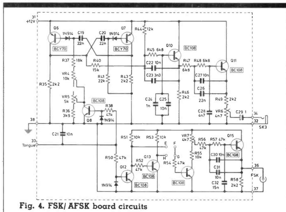
Fig. 4. FSK/AFSK board circuits
