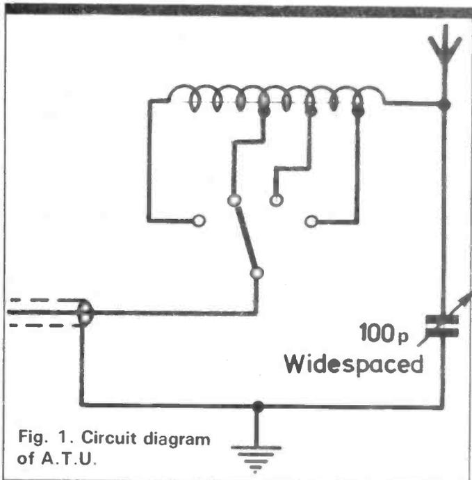
Fig. 1. Circuit diagram of A.T.U.
