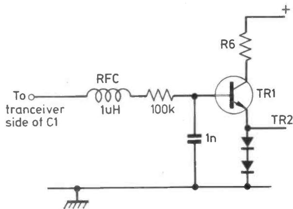
Fig. 5. Modification for full switching with the FT290
