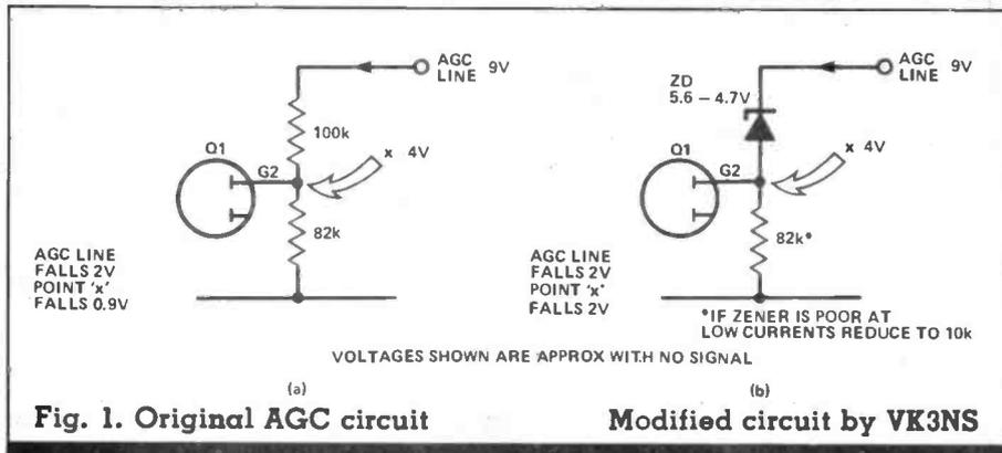
Fig. 1. Original AGC circuit
