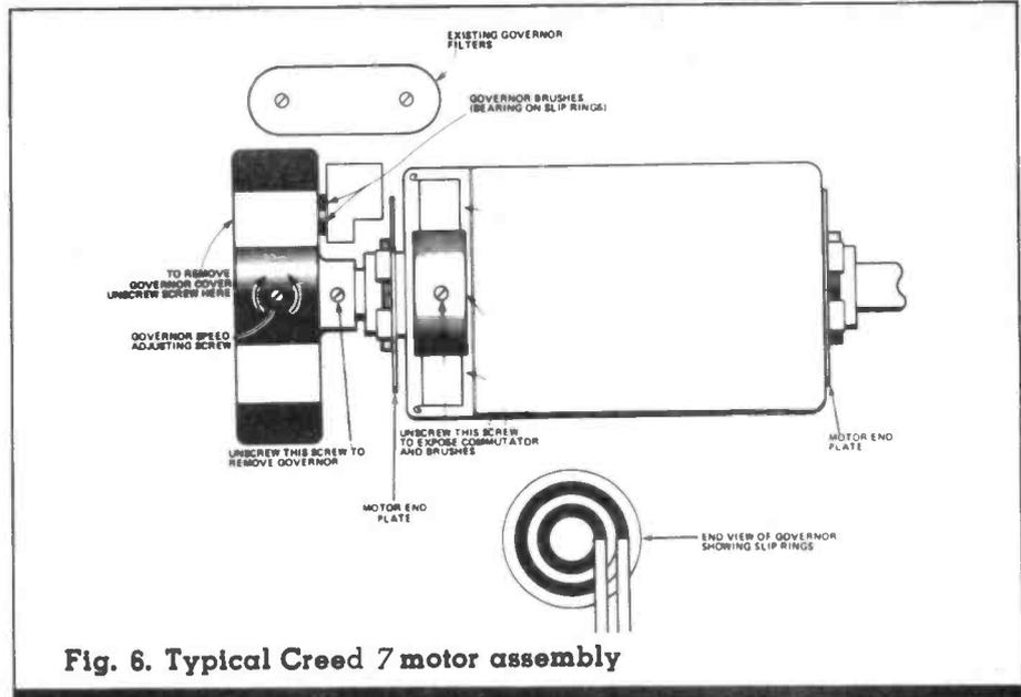
Fig. 6. Typical Creed 7 motor assembly
