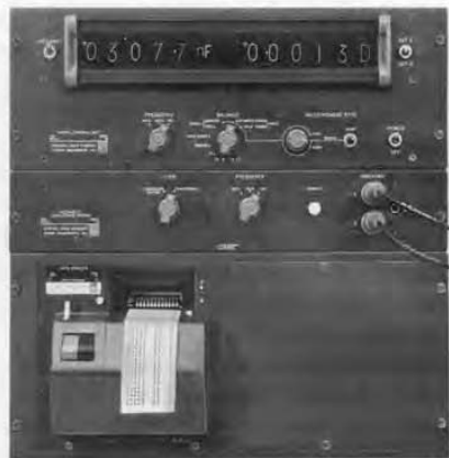
Figure 8. Type 1137-A Data Printer rack-mounted with the automatic bridge.
