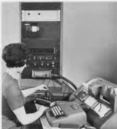
Fig. 9. IBM Model Printing Summary Punch operating from output of automatic bridge. Capacitance values are automatically punched; operator adds serial numbers. Also in relay rack are data printer and (top) intercoupler required for parallel-to-serial conversion.
