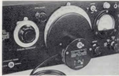
(Above) View of the Type 908-P1 Synchronous Dial Drive installed on a Type 1304-B Beat-Frequency Audio Generator. (Below) Record of the frequency response of a small loudspeaker in an anechoic chamber. Oscillator was driven by the Type 908-P1 Synchronous Dial Drive.
