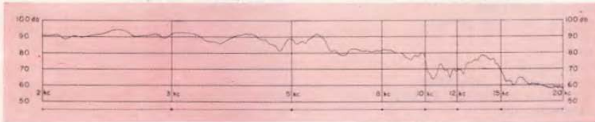
(Above) View of the Type 908-P1 Synchronous Dial Drive installed on a Type 1304-B Beat-Frequency Audio Generator. (Below) Record of the frequency response of a small loudspeaker in an anechoic chamber. Oscillator was driven by the Type 908-P1 Synchronous Dial Drive.
