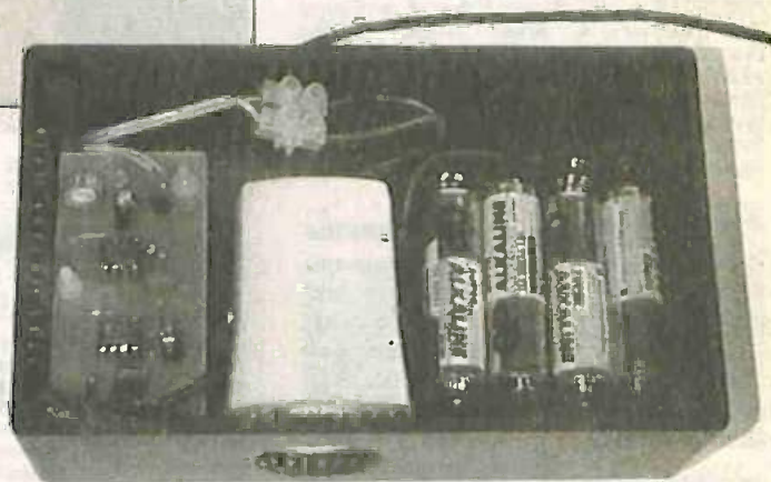
Layout of components in the main unit. Note the siren sound exit hole, 2-way terminal block and battery holder.
