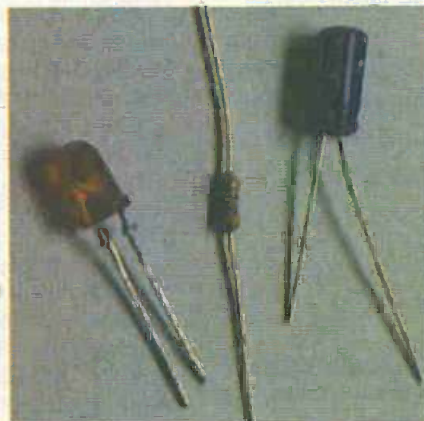
Photo 1.3. Left to right: Light emitting diode, resistor, electrolytic capacitor.
