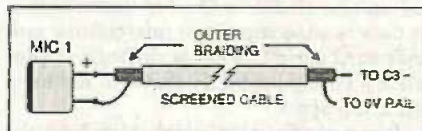
Fig.3. Screened microphone cable must be used if it is more than a few centimetres long.
