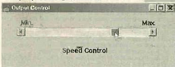
Fig.2. This scrollbar uses one program line to provide control of the printer port.
