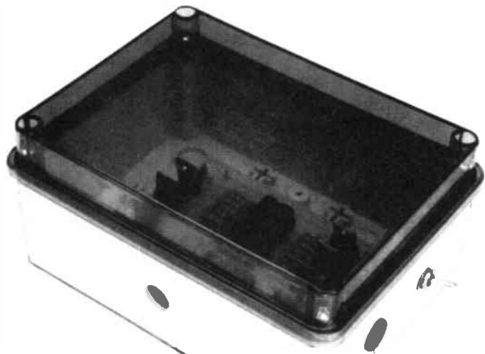
The completed Receiver housed in a case with a transparent lid. A larger case may be required if "switching" relays are to occupy the same case.
