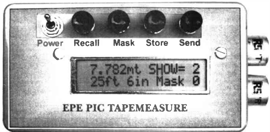
Front panel display window and function buttons. A recalled measurement is shown.
