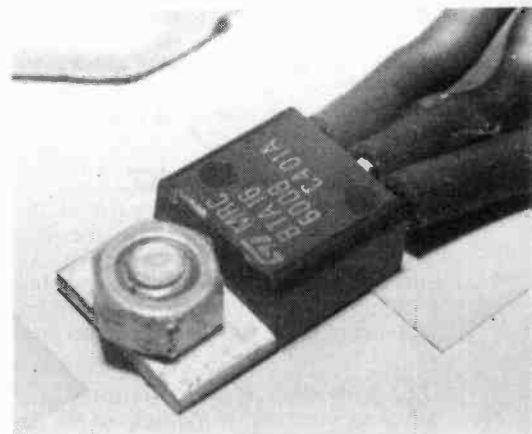
The metal front panel acts as the triac heatsink. Insulating tape under the sleeved pins provides extra protection.
