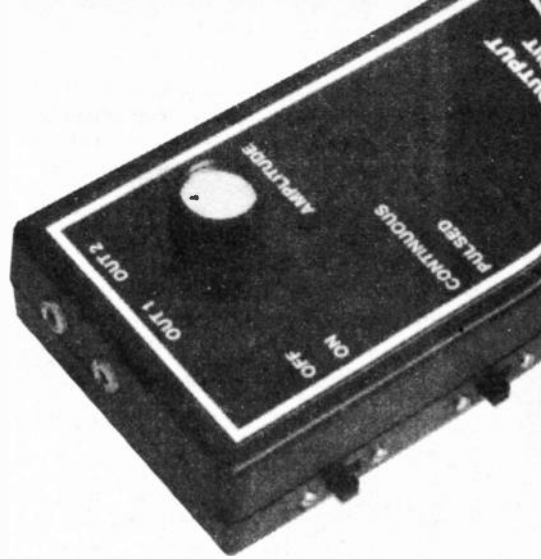
Positioning of the output sockets, i.e.d. and slide switches on the finished unit.
