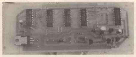
Component layout on completed circuit board. The power MOSFET TR1 has been carefully bent horizontally with the p.c.b.
