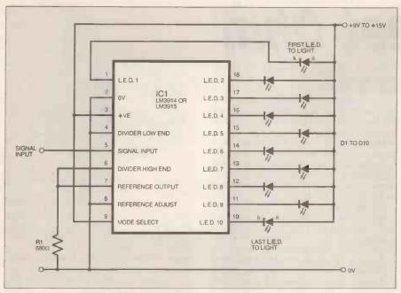
Fig. 8.9. Basic circuit diagram for a bargraph display.
