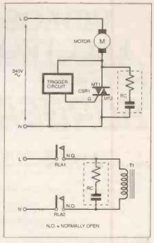
Fig. 3. Typical RC snubber applications
