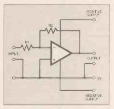
Fig. 8.3. Circuit diagram for an op.amp inverting amplifier.
