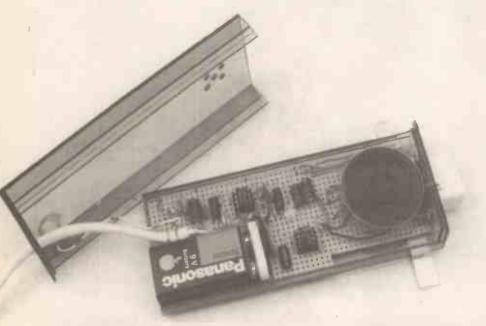
Prototype stripboard version mounted inside the specified case, with transparent lid. Note the positions of the microphone and buzzer.
