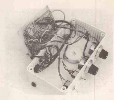
may be more convenient to just use three connections to the p.c.b. and connect the phono sockets, Left with Left, and Right with Right with short insulated wire links, as shown in Fig. 3. Since the two sockets are connected in parallel it is immaterial which are called "input" or "output".
