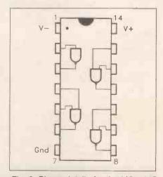
Fig. 3. Pinout details for the MC1488P quad line driver.
