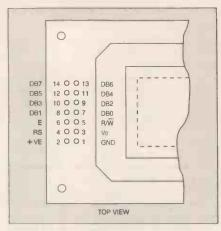
Fig. 4. Pinouts for the I.c.d. module.
