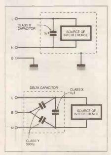
Fig. 4. Suppressor capacitors help prevent interference generated by equipment, feeding into the mains supply, and reduce electromagentic interference.
