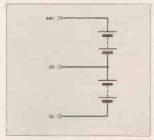
Fig. 8.2. A dual-rail supply formed from two batteries.
