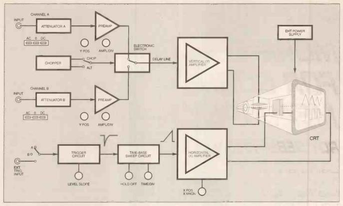
Fig. 2. Block diagram of an analogue dual-trace oscilloscope, excluding focus and brilliance controls.
