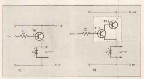
Fig. 8.210. Two examples of a pnp switch: (a) a single transistor and (b) a Darlington transistor.
