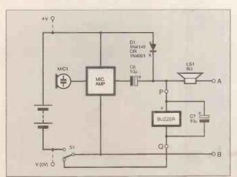
Fig. 3. Telephone with automated calling. The line connects A and B to the same points on the distant phone. When the phone is not in use, the gravity switch S1 adopts the position shown. For the dotted connections see the text.
