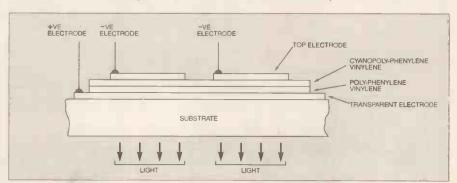
Fig. 1 The structure of a light emitting polymer display.
