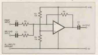
Fig. 8.5. Basic 2-channel op.amp mixer circuit.
