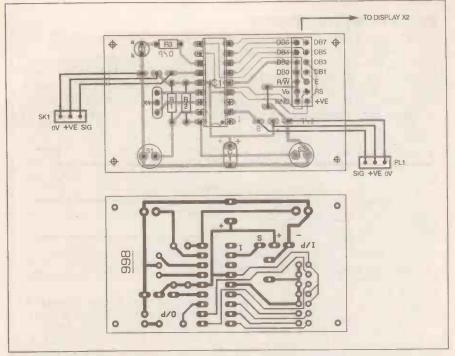
Fig. 3. Printed circuit board component layout and full size copper foil master track pattern for PulStar.
