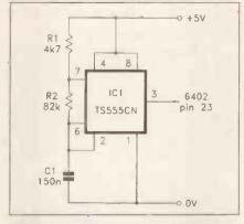
Fig. 5. A circuit which provides regular triggering to the 6402 UART.
