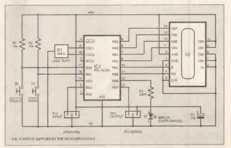
Fig. 2. Complete circuit diagram for PulStar.
