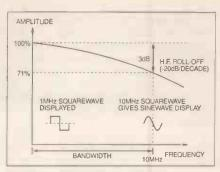
Fig. 8. Frequency response of a 10MHz oscilloscope.
