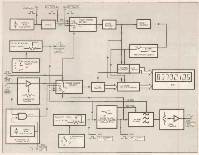
Fig. 1. Block diagram for the Ultra-Fast Frequency Generator and Counter.
