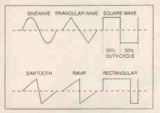
Fig. 6. Idealised standard waveforms.
