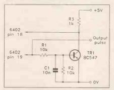
Fig. 1. Circuit which generates a strobe pulse each time a fresh byte of data is available.
