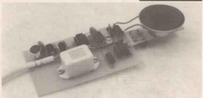
The first prototype phone built on a printed circuit board. This prototype was not intended to be housed in a case so the microphone and buzzer were mounted directly on the p.c.b. When inserted in the case, the p.c.b. has to be cut to take the battery, the microphone mounted inside the lid and the buzzer on the outside of the case.
