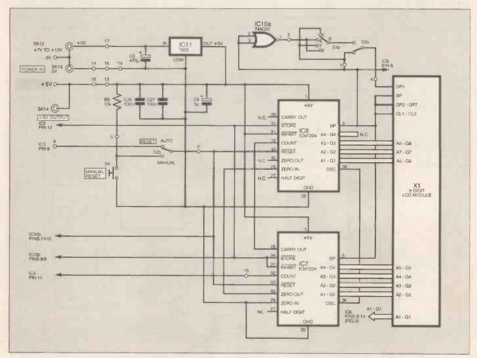
Fig. 4. Circuit diagram for I.c.d. digits 2 to 7 counter/driver, display and power supply.
