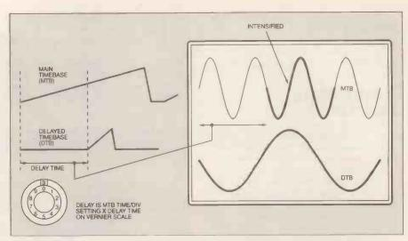
Fig. 10. Delayed timebase showing expanded display of main timebase.
