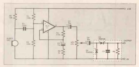
Fig. 8.4. Circuit diagram for the audio input module which produces a d.c. output voltage relative to the input signal amplitude.
