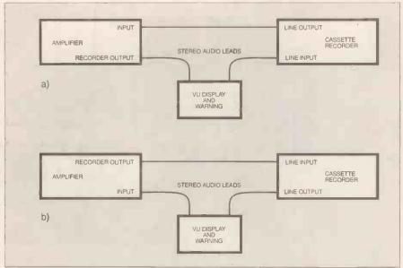
If the connection method shown in Fig. 4a is used, then any adjustment of the gain setting on the recorder must be copied on VR2. Whichever connection method is used, the original signal is not processed in any way by the project. Although the unit does impose an additional load of about  $10 \mathrm{k}\Omega$  on the signal source, normally this should be of no significance.
