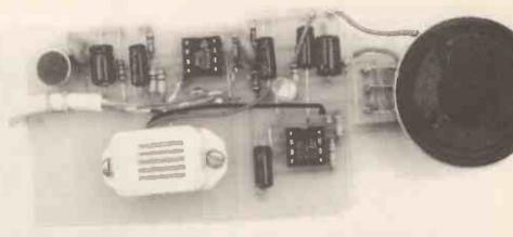
The microphone insert and buzzer are not mounted on the p.c.b. in the final version. The board is carefully cut to make space for the battery and the microphone is glued to the inside lid of the case – see below.
