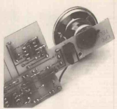
The lever-operated microswitch is mounted on the copper track side of the p.c.b. The pole (p) of the switch connects to line B. Note the position of the loudspeaker.
