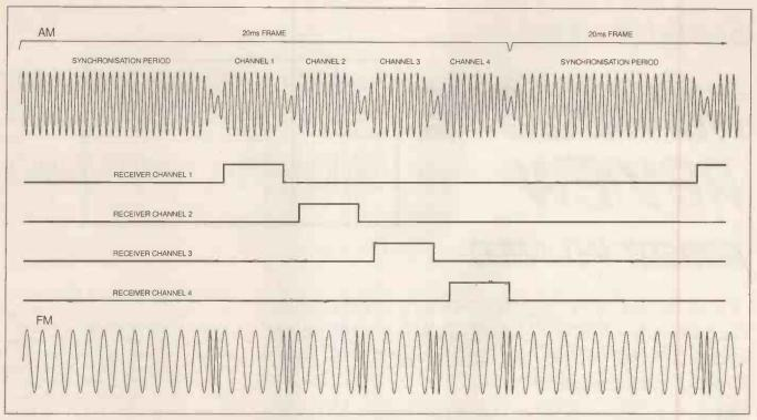
Fig. 6. Comparative waveforms generated by AM and FM systems to control four receiver channels.
