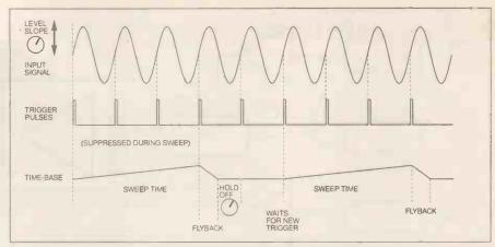
Fig. 4, Timebase generator output waveforms.
