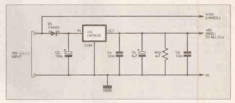
Fig. 2. Supply voltage regulation circuit for the i.c.s.
