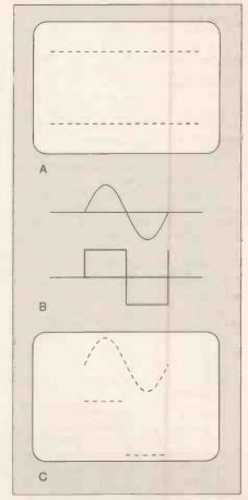
Fig. 3. Timebase presentation of signals on a dual-trace oscilloscope.
