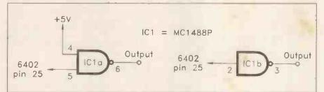
Fig. 4. Using the driver in the MC1488P.
