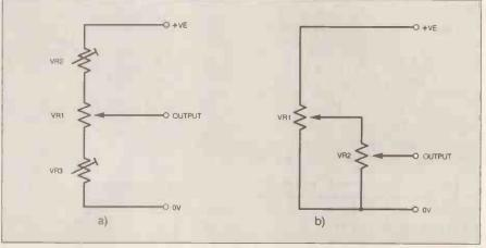
Fig. 8.8. Two methods for restricting the output voltage range from a potentiometer.
