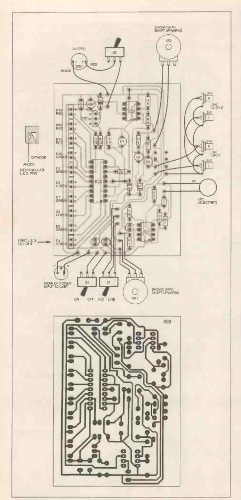
Fig. 3. Printed circuit board component layout and full-size underside copper foil track master pattern.
