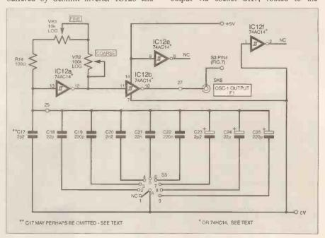
Fig. 2. Circuit diagram for Oscillator-1.
