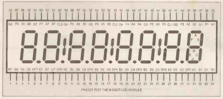
Fig. 8. Pinouts for the 8-digit I.c.d. module and (right) the ICM7224 counter/driver.
