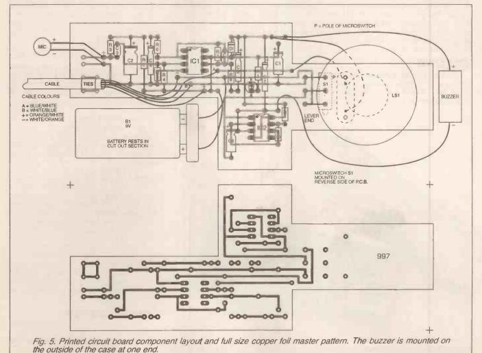
respecting polarity, solder these wires to their copper pads on the p.c.b. Temporarily connect the buzzer.
