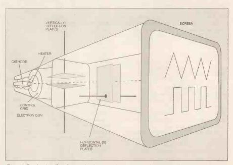
Fig. 1. Basic details of a cathode ray tube as used in an oscilloscope, excluding focussing and acceleration anodes.
