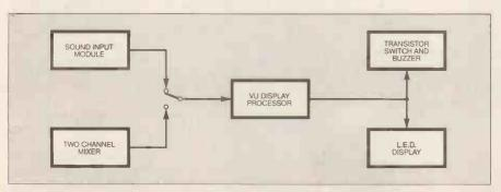
Fig. 1. Block diagram for the VU Display and Alarm.
