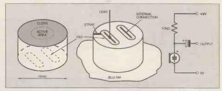
Fig. 2. Condenser (electret) microphone. The negative terminal is identified by the strap which connects it to the case. Two pads are provided for leads. These are loaded with solder, which conceals the internal connections shown. To solder a lead, press the mike into some Blu-tack. Then melt the solder on the pad, and stand a vertical wire outside the internal connection, as drawn. To lift the mic. from the Blu-tack, rock gently. Output is taken from a series resistor, as indicated.
