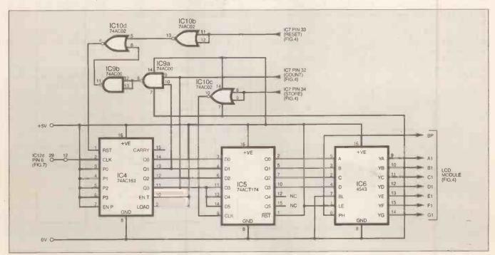
Fig. 5. Circuit diagram for I.c.d. digit 1 counter/driver.
