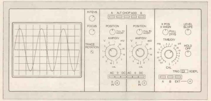
Fig. 5. Stylized layout of the basic controls on a typical dual-trace oscilloscope.
