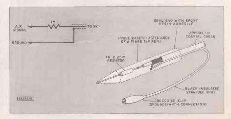
Fig.8. Input probe
