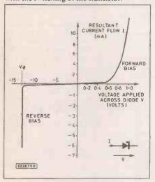
Fig. 2. Zener diode characteristics.
