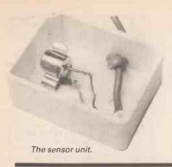
Make the sensor connections (polarity unimportant). Excessive heat should not be applied so soldering should be done quickly. Secure the switch in the clip and attach the lid. Solder the "power in" type connector to the other end of the sensor connecting wire and fit the blanket with the correct type of plug for SK2.
