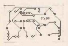
3.16 P.C.B. layout for TBA820M power amplifier module
