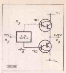
Fig. 3.7 Complementary output stage based on power Darlington transistors
