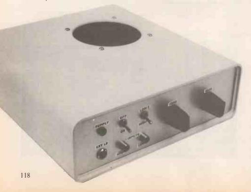
HEN bench testing audio and radio equipment, one often realises the need for a means of listening to the signals which are present in the various stages under examination. In order to examine signals in this way, all that is required is an audio frequency amplifier and loudspeaker together with a means of attachment to the equipment under test.
