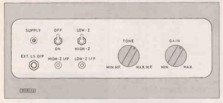
Fig. 4. Recommended front panel layout
