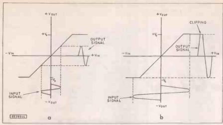
Fig. 3.2(a) Effect of Fig. 3.1 on a sinusoidal input signal of moderate amplitude Fig. 3.2(b) Effect of Fig. 3.1 on a sinusoidal input signal of large amplitude (amplifier being over-driven)
