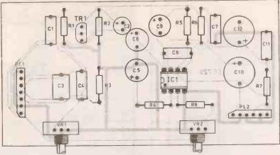
Fig. 3. P.C.B. copper foil and component layout
