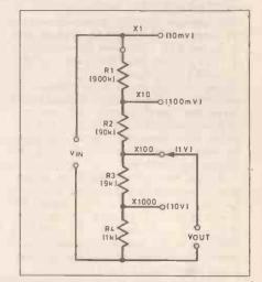
Fig.3. (a) Step attenuator for millivoltmeter, with resistance values for an impedance of one megohm.
