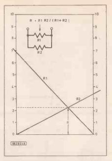
Fig. 1. Parallel resistance calculator. The lines between 0 and R1, 0 and R2 intersect at a height which gives R.
