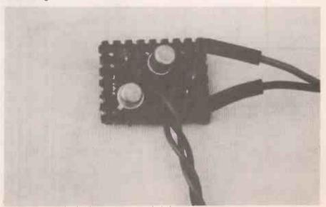
Before soldering, the usual preparations to the copper tracks should be made, making sure they are cleaned of any oxide, a clean-up of the soldering iron tip is useful too. This improves the speed and quality of the solder joints, prevents damage to the active components by overheating, and improves the reliability of the finished product.
