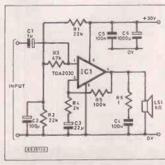
Fig. 3.20 TDA2030 power amplifier (single supply)
