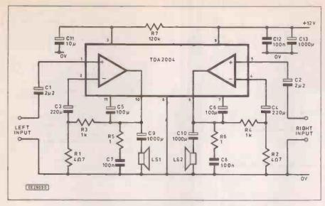
Fig. 3.18 TDA 2004 stereo power amplifier
