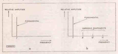
Fig. 3.3(a) Frequency spectrum associated with the output signal in Fig. 3.2(a) Fig. 3.3(b) Frequency spectrum associated with the output signal in Fig. 3.2(b)
