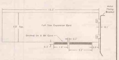
Fig. 2. Basic mechanical details of a full length PC expansion card.
