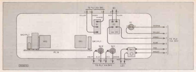
Fig. 5. Internal wiring of the Bench Amplifier/Signal Tracer
