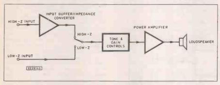
Fig. 1. Block diagram of the Bench Amplifier/Signal Tracer
