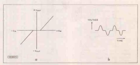
Fig. 3.5(a) Magnified version of Fig. 3.1 at the zero axis crossing point Fig. 3.5(b) Effect of Fig. 3.5(a) on a signal of low amplitude
