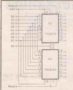
Fig. 1. Simple circuit for providing 8-bit input and output ports for use with the address decoder circuits provided last month.
