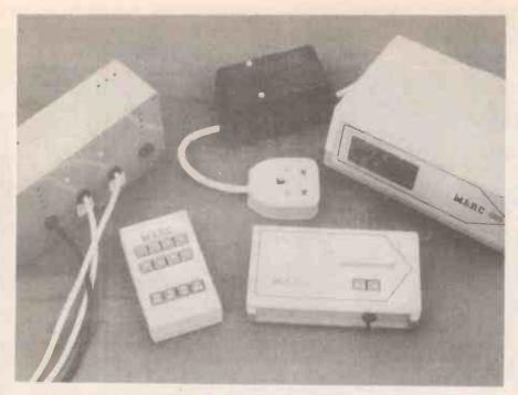
The line-up of already published MARC control system units showing, from left to right, temperature mains interface, decoder, encoder, handheld infra-red transmitter and temperature display. Next month a Pocket DTMF Tone Generator will be described.
