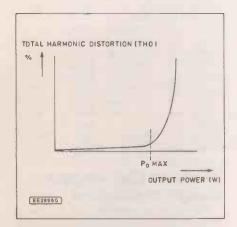
Fig. 3.4 Relationship between total harmonic distortion and output power (note the onset of clipping)
