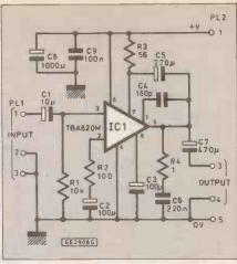
Fig. 3.15 TBA820M power amplifier
