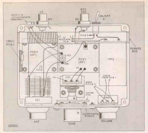
Fig. 8. The completed receiver showing board positioning and wiring to support hardware (full size).
