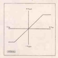
Fig. 3.1 Transfer characteristic for a typical power amplifier
