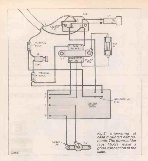
the circuit panel to the base of the box using short fixings and stand-off insulators. Make certain that all connections on the copper track side of the panel remain well clear, at least 4mm, of the case bottom. Place a piece of thick cardboard between the board and metalwork.
