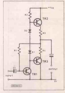
Fig. 3.9 Basic circuit of a practical complementary power amplifier
