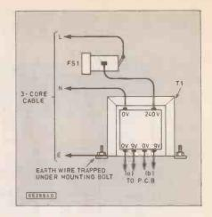
Fig. 5. Wiring details for the mains transformer T1.
