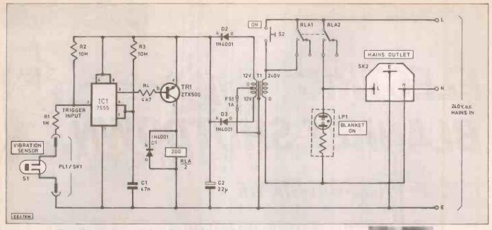
Fig. 1. Circuit diagram of the Electric Blanket Shut-Down.
