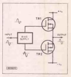
Fig. 3.8 Complementary output stage based on power MOSFET transistors
