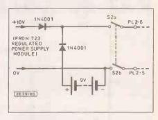
Fig. 7. Modifications for dual mains/ battery operation
