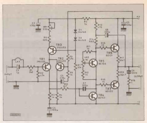
Fig. 3.11 High quality power amplifier module
