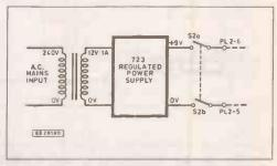
Fig. 6. Modifications for mains operation
