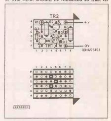
Fig. 3. Component layout and details of breaks required in the underside copper tracks.
