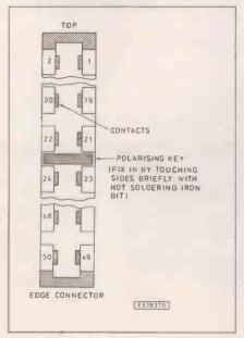
Fig. 3. Polarising key positioning in the Amstrad connector.
