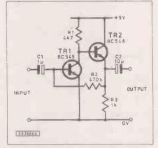
Fig. 2.7. Two-stage amplifier with lowimpedance output
