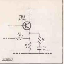
Fig. 2.12. Modification to the general purpose transistor amplifier module in order to permit gain setting
