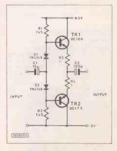
Fig. 2.15. Low-power complementary output dirver for use with low impedance loads.
