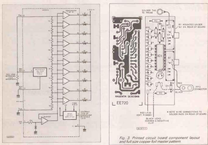
Fig. 2. Internal circuit details for the LM3914N i.c.
