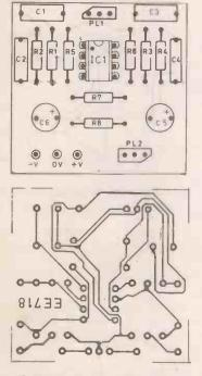
Fig. 2.21. P.C.B. layout for the general purpose operational amplifier module
