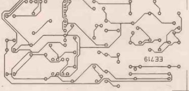
Fig. 5. P.C.B. layout for the simple intercom.
