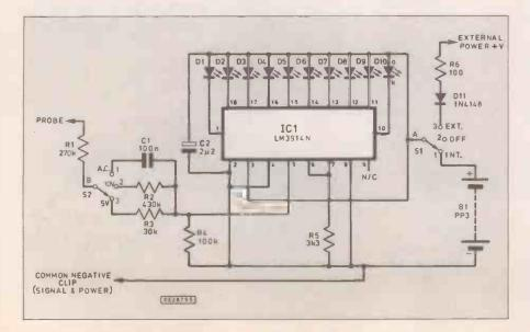
were tried. Some were cheaper, but needed much more p.c.b. space and were more complicated. Using the LM3914N gives several other benefits. It has a stable internal reference voltage, programmable l.e.d. current, and a high input impedance. It is also very tolerant of overloads.
