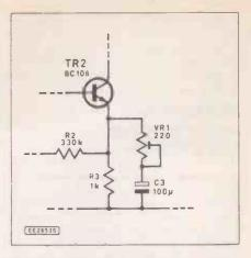
Fig. 2.13. Modification to the general purpose transistor amplifier module in order to permit variable gain adjustment
