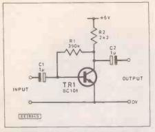
Fig. 2.3. Simple common-emitter amplifier stage
