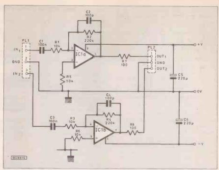
Fig. 2.20. Circuit diagram of the general purpose operational amplifier module
