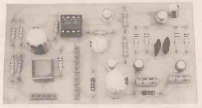
tors, capacitors, diodes and transistors. As with all of our projects, it is impor-tant to ensure that all of the components are correctly located. Furthermore, in the case of the polarised components (such as electrolytic capacitors, diodes and transistors) it is absolutely essential to ensure that each component is correctly orientated.
