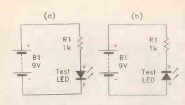
Fig. 3. Simple I.e.d. polarity test circuit. If the I.e.d. lights it has the polarity shown in (a), if not he polarity is as shown in (b).
