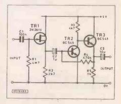
Fig. 2.9. Adding an f.e.t. input stage to obtain a very high input impedance
