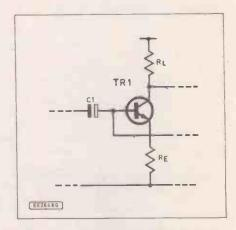
Fig. 2.8. Modification to Fig. 2.7 to permit gain setting by negative feedback
