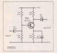
Fig. 2.6. Emitter stabilised commonemitter amplifier stage
