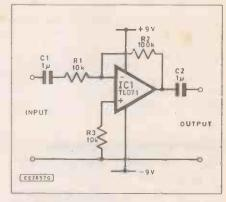
Fig. 2.17. Practical inverting amplifier
