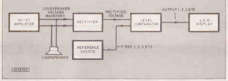
Fig. 1. Spatial Power Display block diagram and waveforms (below) showing the basic principle of operation
