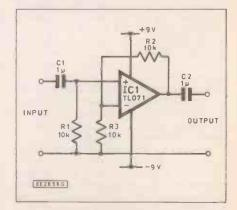
Fig. 2.18. Practical non-inverting amplifier
