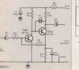
Fig. 2.11. General purpose transistor amplifier module
