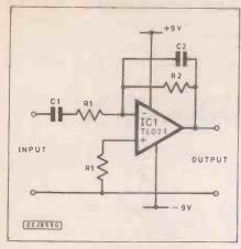
Fig. 2.19. Bandwidth limited inverting operational amplifier
