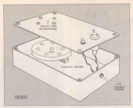
Fig. 4. Guide to the layout of components inside the small plastic case. The microphone insert sits above IC1 and is held in place with a piece of Blutack.
