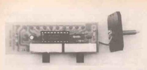
The completed circuit board with the slide switches soldered in position. Resistor R1 is mounted track side – see photo below.
