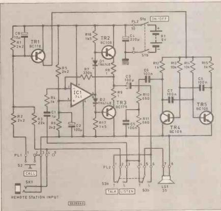
Fig. 3. Complete circuit diagram of the simple intercom.
