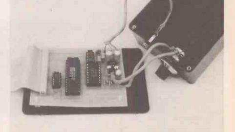
Prototype of the sound generator p.c.b.. In this verison the AY-3-8913 was used.
