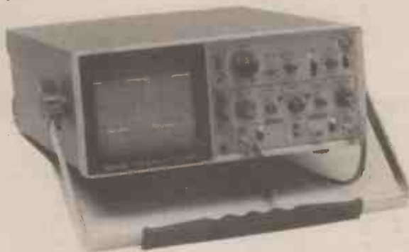
V212 DC-20MHz, 1mV/div, dual channel . . . . . £385.00
