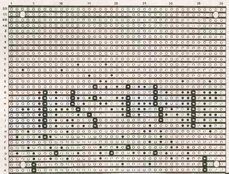
Fig. 4. Stripboard component layout and details of breaks required in the underside copper tracks.
