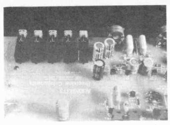
Close-up view of the p.c.b. push-button input mode selection switches.
