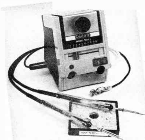
The Antex TCSU1 soldering station has an anti-static earth connection to protect MOS devices. The temperature can be pre-set anywhere between 65 and 430 degrees centigrade. Three iron-coated bits are also supplied with each station. Priced at £90.22 (inc. p & p). Antex (Electronics) Ltd. , Mayflower House, Plymouth, Devon. ☎ 0752 667377.
