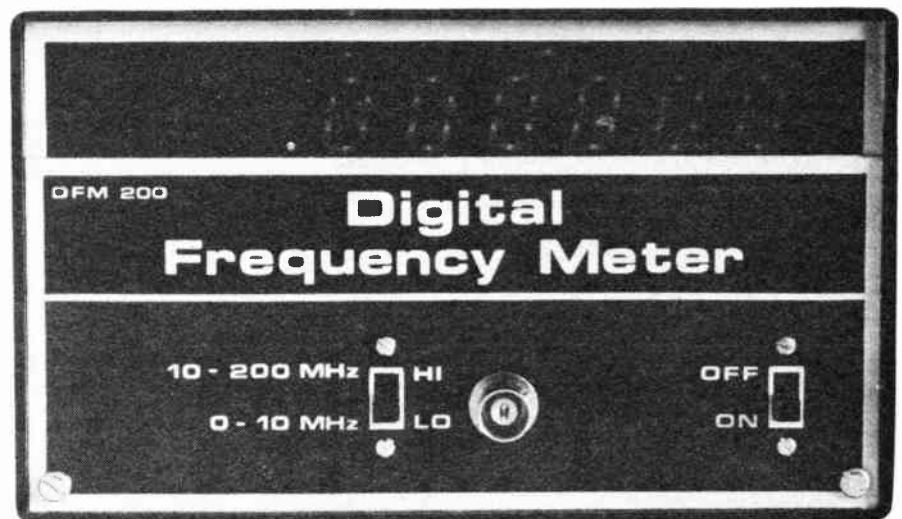
Front panel layout and legend for the 200MHz Digital Frequency Meter.
