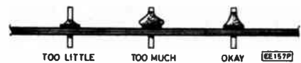
Fig. 10. Identifying the correct amount of solder to apply is a matter of common sense and, of course, practise.
