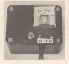
preserving readings below 1V approximately since any such cell would be "dead" Similarly, with 9V batteries, the section of scale below 6V is not needed. This maximises the useful part of the scale and leads to more accurate readings. A slide switch selects a basic load according to whether a 1.5V or a 9V battery is being tested and a push-button switch increases the load by a factor of five for larger types of battery.
