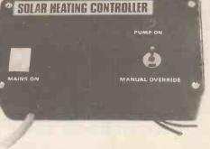
mal efficiency. The controller described here can be used for most solar heated water systems. It ensures that water is pumped only when there is a useful amount of heat to be gained.
