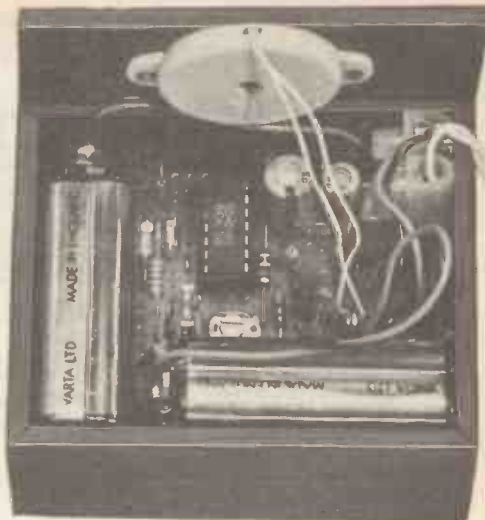
View showing the layout of the circuit board and batteries within the case.
